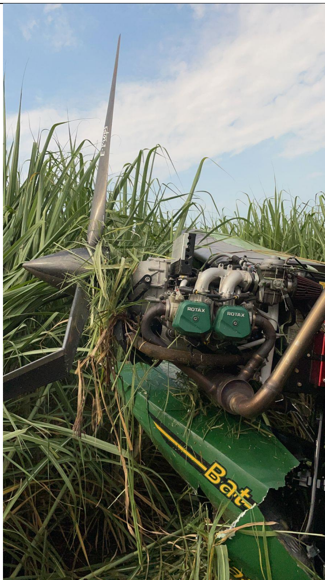
Figure 3: The damaged airframe and propeller blade. (Source: Operator)
