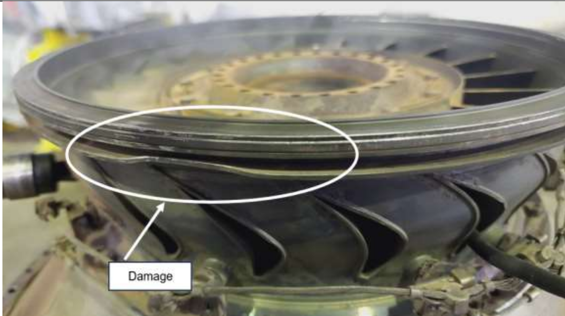
Figure 4: The damaged outer casing.
