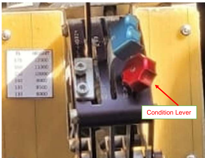
Figure 3. The quadrant with the condition lever moved backward. (Source: Operator)
