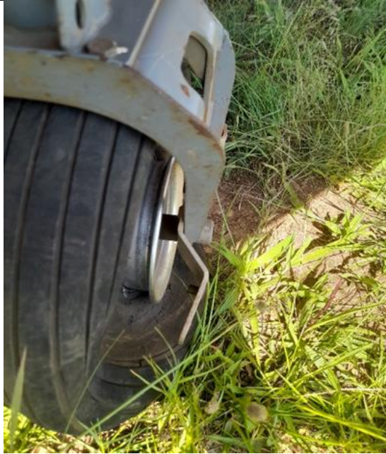
Figure 3: The burst nose wheel tyre. (Source: Operator)
