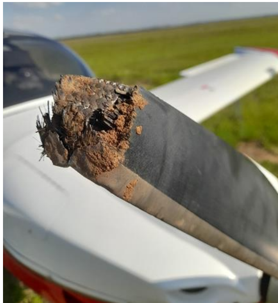
Figure 4: Damage on the propeller blade tip. (Source: Operator)
