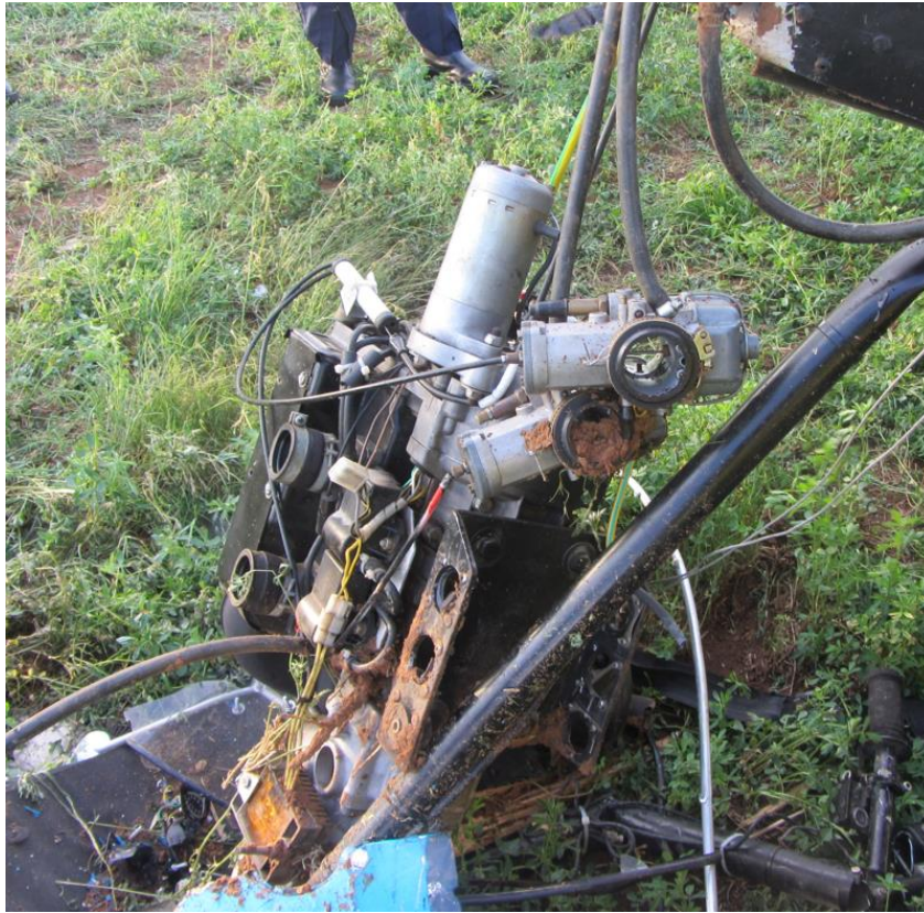
Figure 11: The engine with soil and dirt on the front surface.
