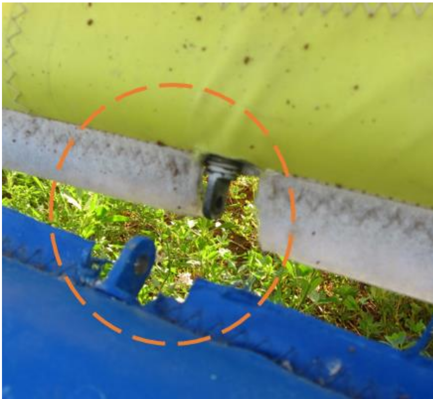
Figure 9: The orange circle shows the second unsecured attachment point of the left aileron.
