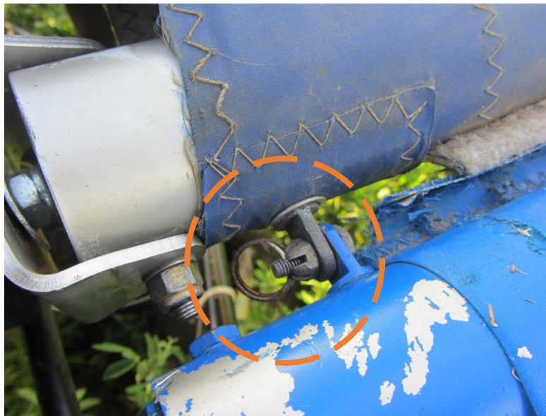
Figure 8: Right-side aileron attached with a bolt, nut and safety ring.
