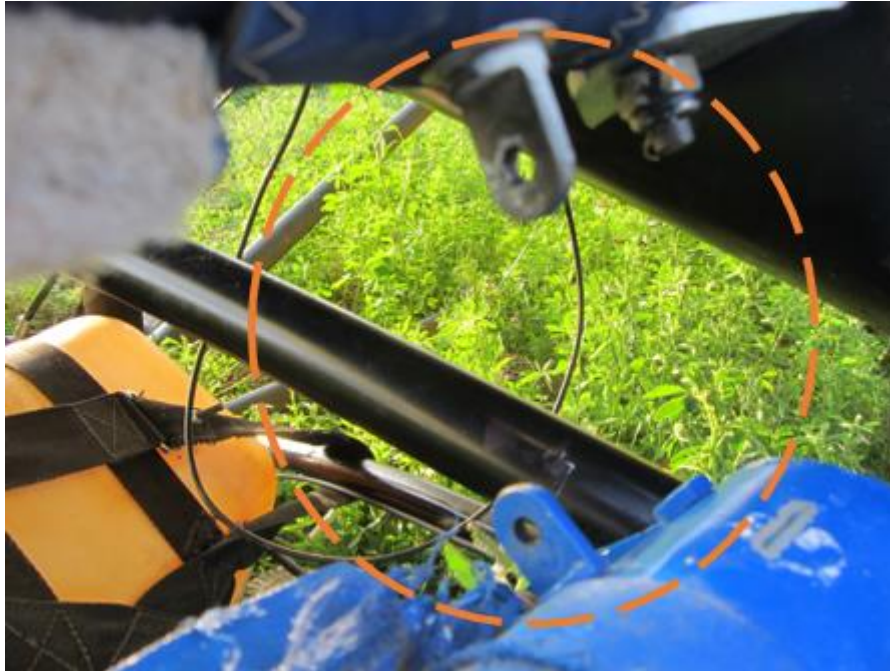
Figure 7: The orange circle shows the unsecured left aileron inboard attachment points.
