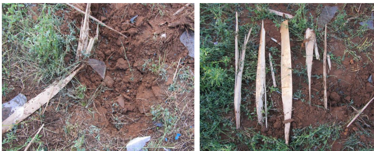
Figure 14 (left and right): One of the fragmented blades was buried on the ground with the hub (left), and the pieces of the fragmented blades spread out on the ground (right).
