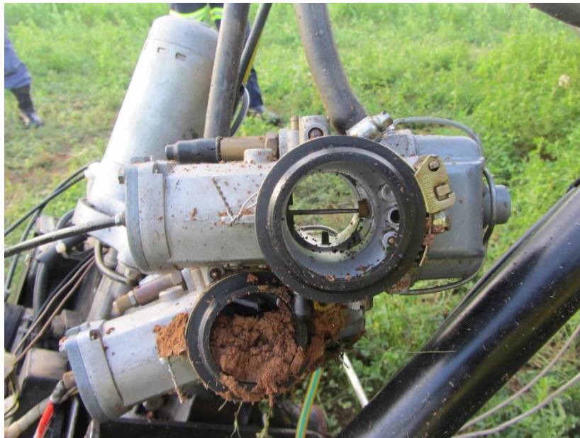
Figure 12: The dislodged carburetors.
