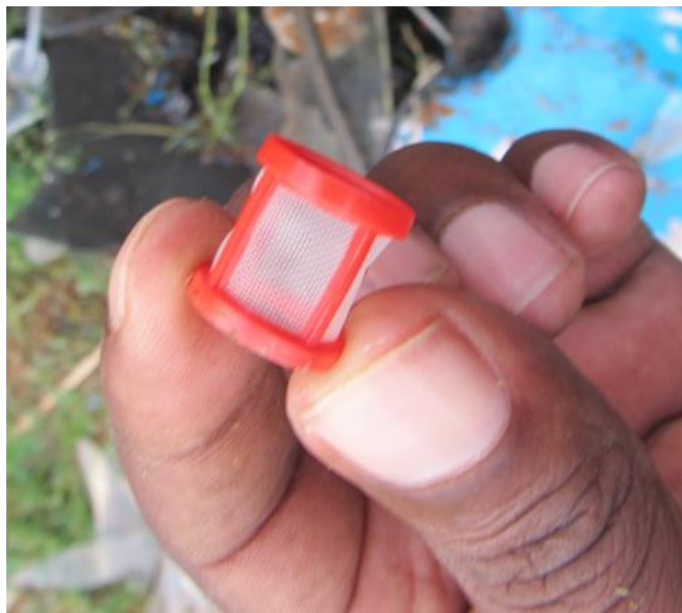
Figure 13: The dirt-free carburetor filter.
