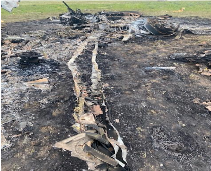
Figure 11: The right wing that was destroyed by the fire.
