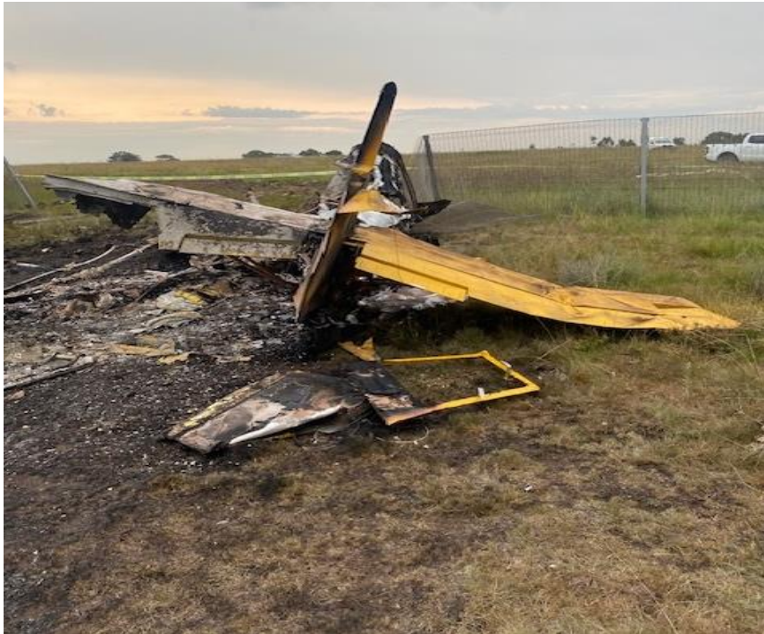
Figure 9: The wreckage facing the direction from which it had approached (south).
