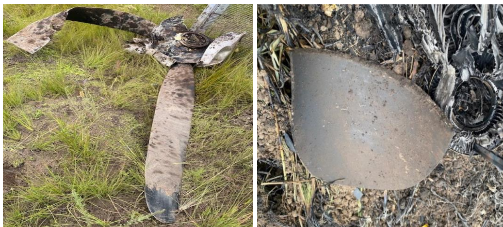
Figures 12 and 13: The propeller that separated from the hub (left); and the blade tip that broke off from one of the blades (right).
