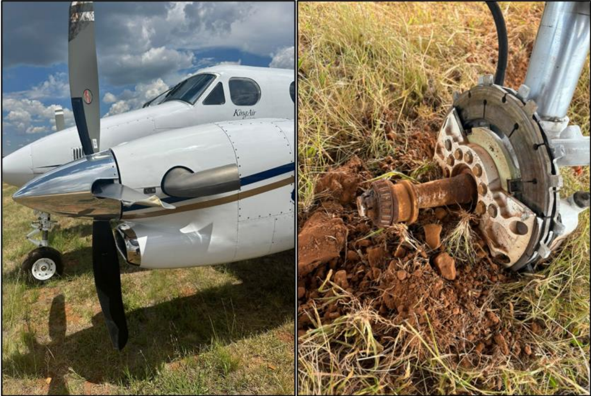
Figures 2 and 3: Damage to the No.1 propeller blades (left) and the left main landing gear axle (right) post-accident. (Source: Pilot)
