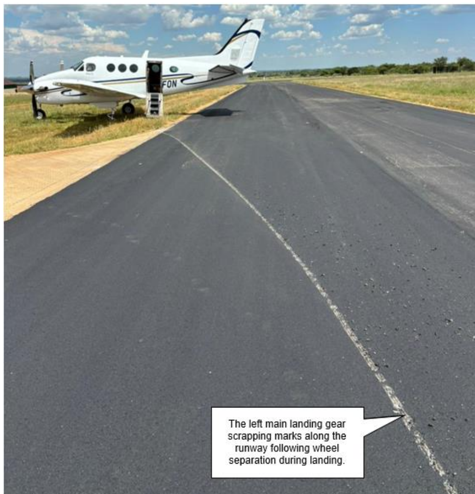
Figure 4: The aircraft after the accident and the scrape marks on the runway. (Source: Pilot)
