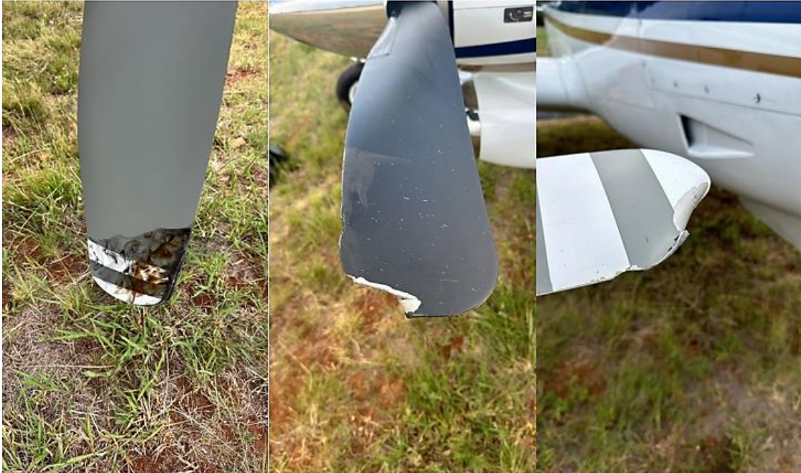
Figures 6, 7 and 8: Tyre material on the blade tip (left), and damage to the two propeller blades (middle and right). (Source: Pilot)
