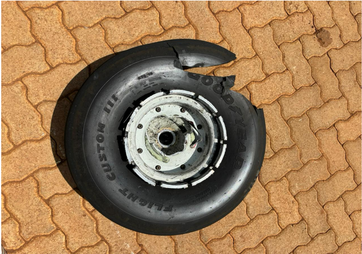
Figure 5: Damage to the left main landing gear inboard hub. (Source: Operator)
