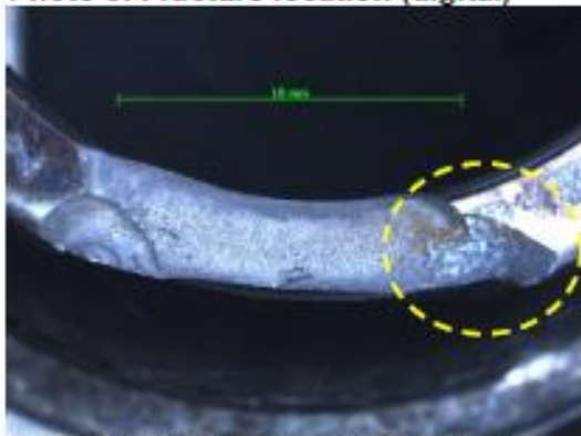
Photo 4: Fracture location (stereo)
