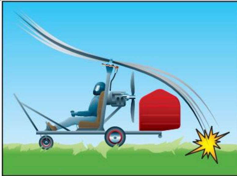
Figure 4: Taxiing too fast or gusting winds can cause the blade to flap if the rotor is turning slowly. If not controlled, the rotor blade could strike the ground. (Source: faa-h-8083-21.pdf )
