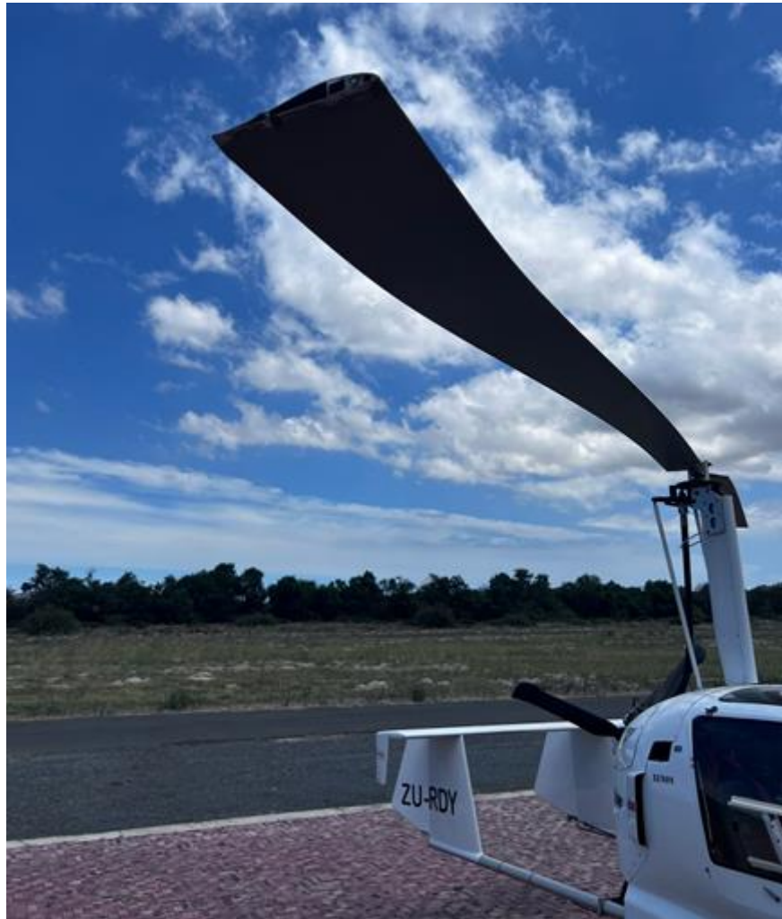
Figure 3: The damaged rotor blade. (Source: Pilot)
