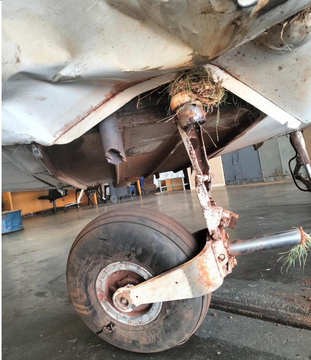
Figure 4: Damage to the nose landing gear oleo and aircraft structure.
