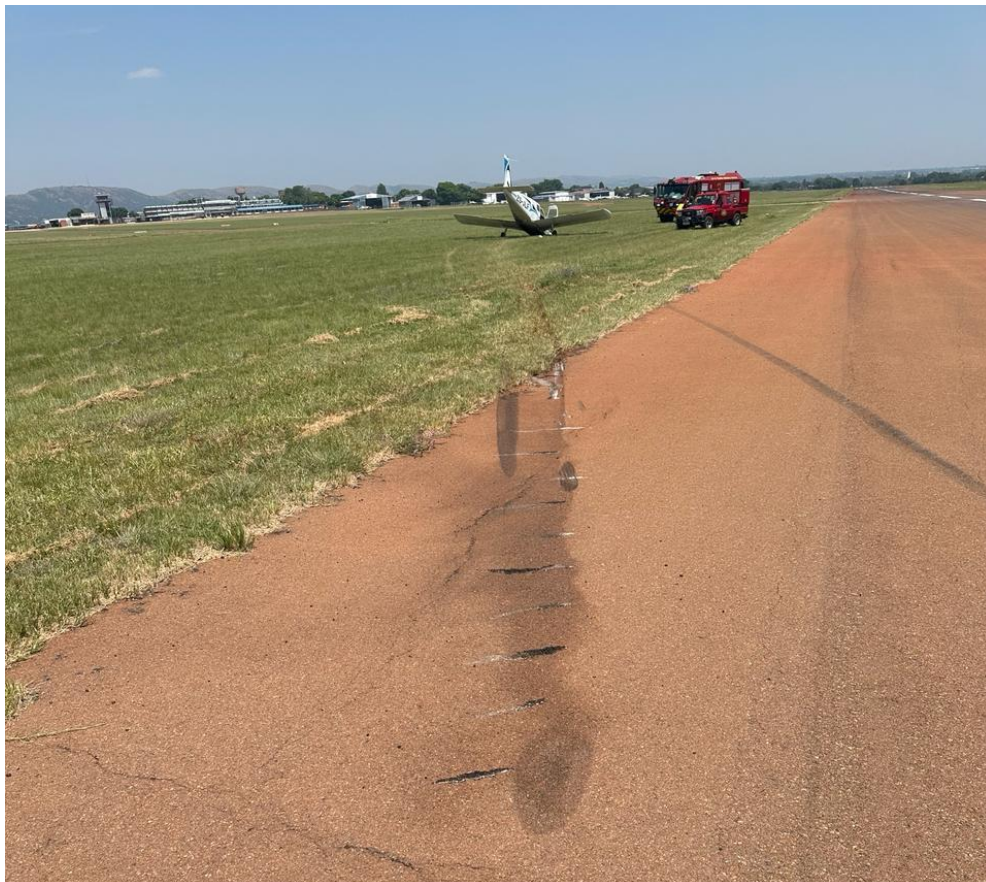
Figure 1: Propeller strike markings on the edge of the runway. (Source: ARFF)
