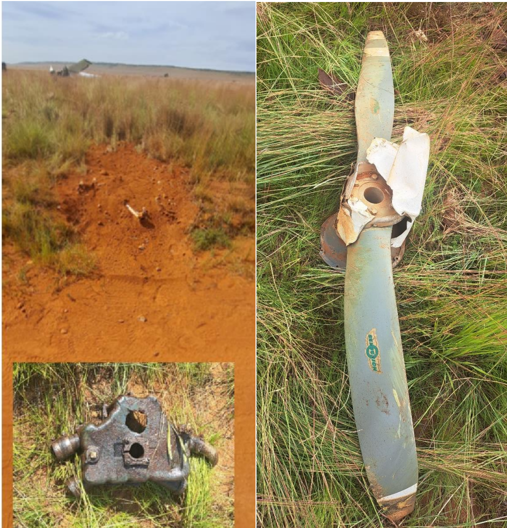
Figure 4: First point of impact (inset: oil reservoir). Figure 5: The twisted propeller indicates a substantial amount of power at impact.
