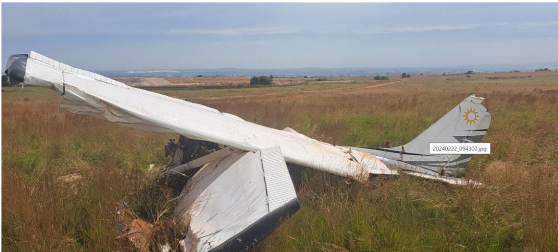
Figure 7: The damage to the top and left side of the right wing.
