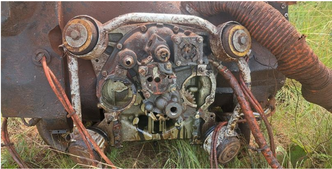
Figure 3: The engine separated from the airframe; the engine mount is still attached.
