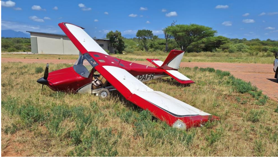
Figure 3: The damaged wing, propeller and landing gear. (Source: Pilot)
