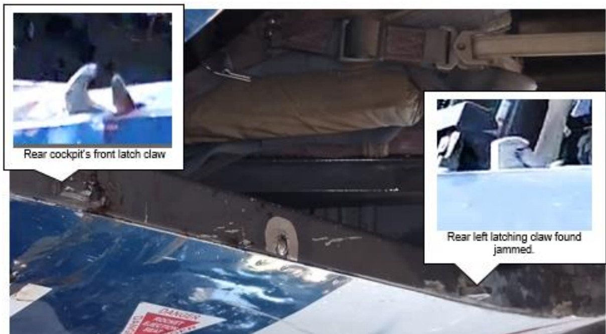
Figure 8: Rear cockpit left-side latch claws after the accident.
