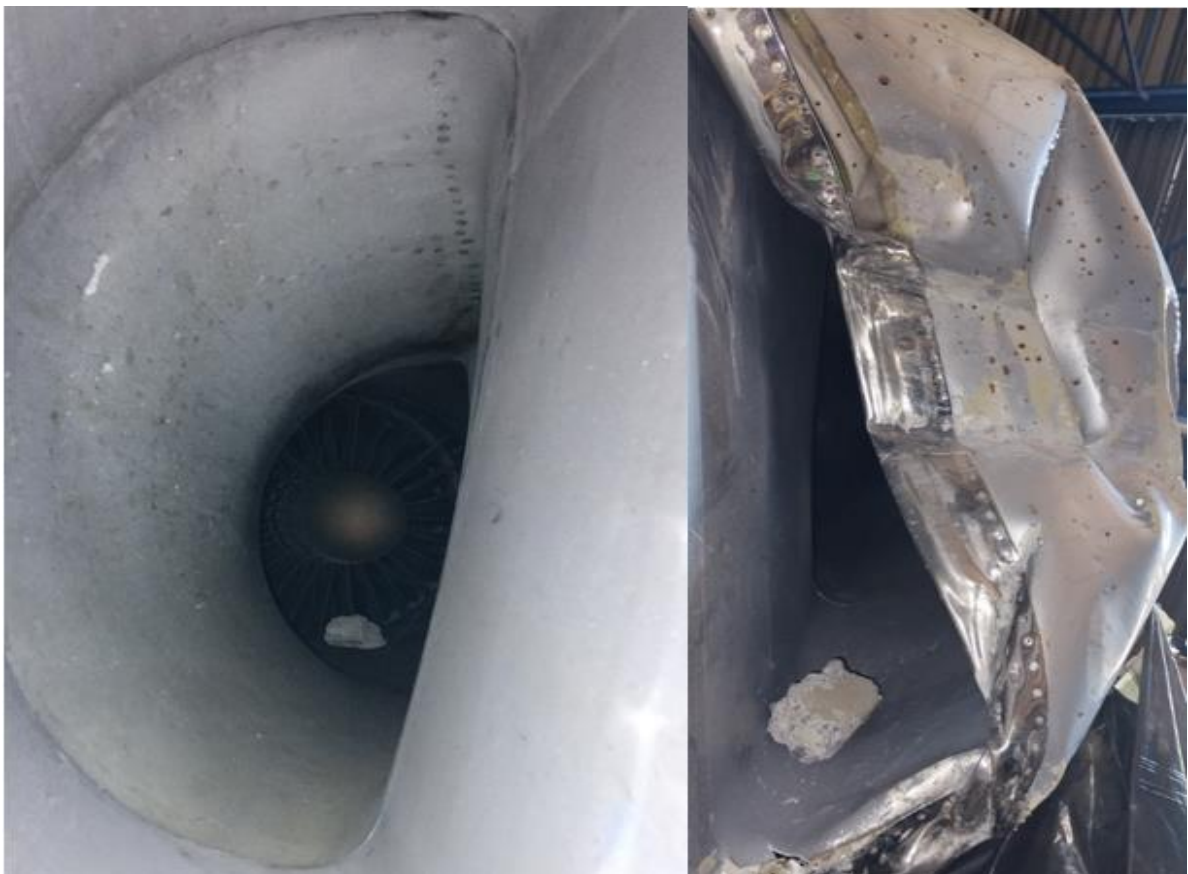
Figure 5: Left- and right-air intake with debris.
