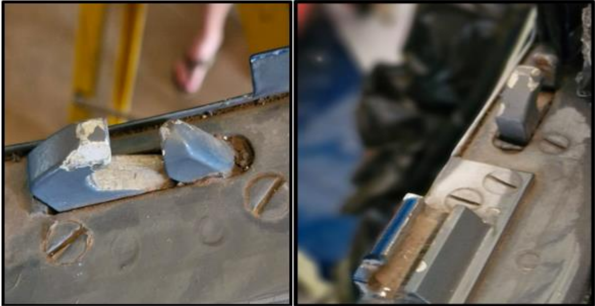
Figure 7: The chipped paint on the top side of both the right front latch claw and rear latch claw of the rear cockpit.
