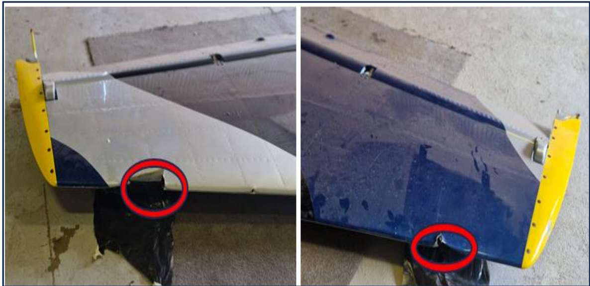
Figure 6: Damage to the horizontal stabiliser with evidence of concrete debris.
