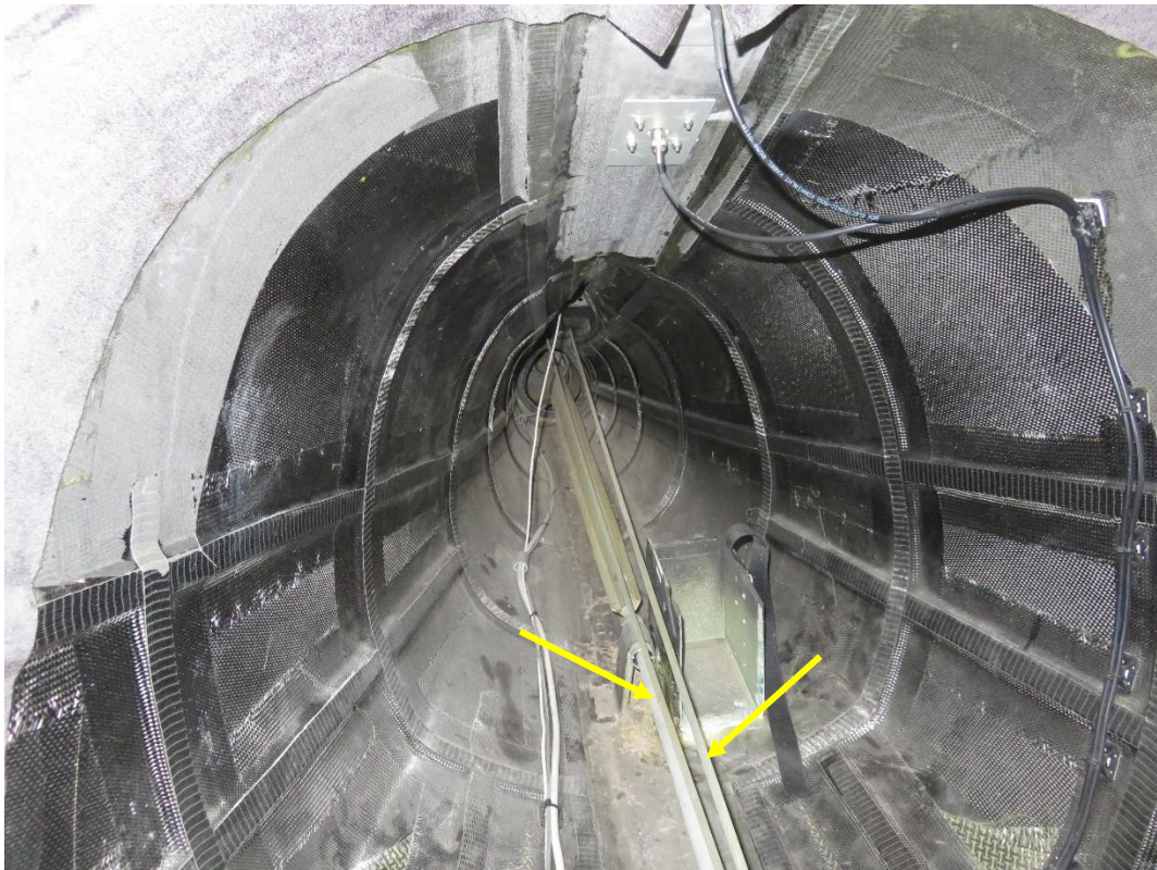
Figure 6: The left and right rudder cables in the boom area of the aircraft were in place and undamaged.
