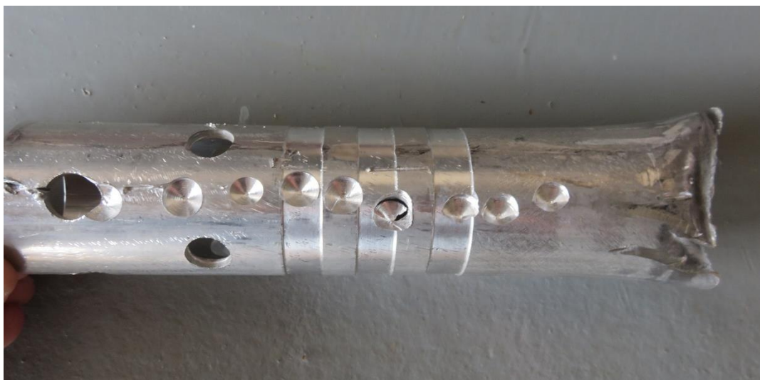
Figure 11: The nose gear strut bottom section with drill holes.
