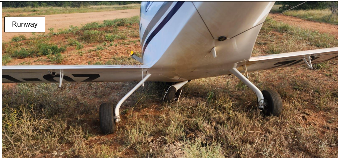
Figure 3: The aft view of the aircraft shows the collapsed nose gear. (Source: Pilot)
