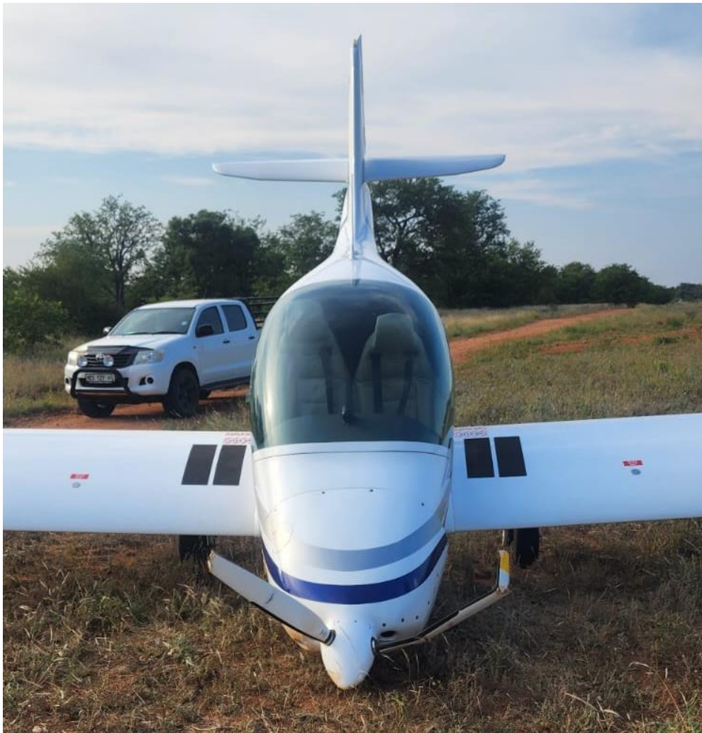
Figure 4: The front view of the aircraft shows the damaged propeller blades. (Source: Pilot)
