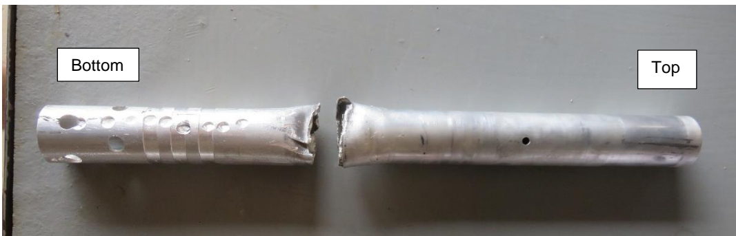
Figure 10: The failed nose gear strut.
