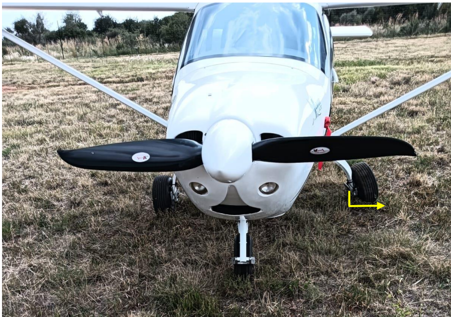
Figure 2: The aircraft at the accident site with the damaged left main gear wheel axle. (Source: Pilot)
