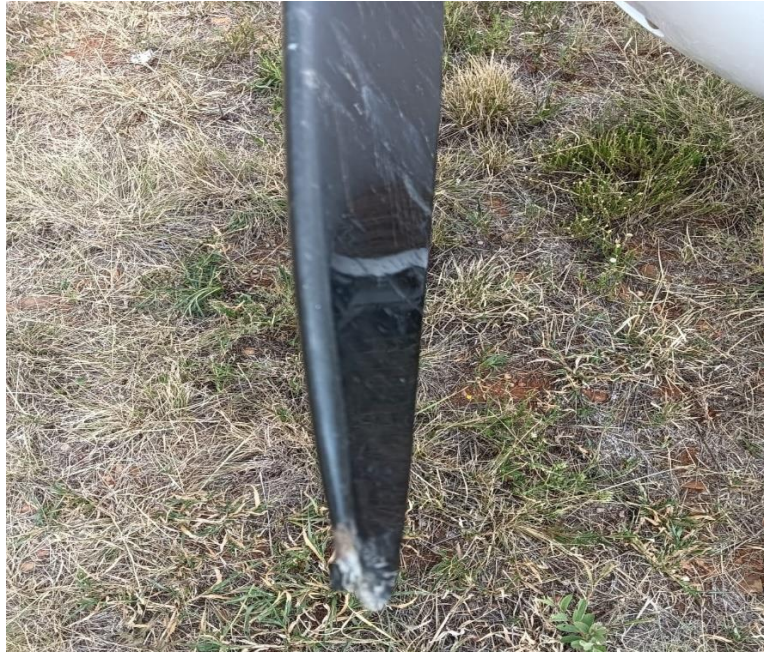
Figure 3: The damaged blade tip. (Source: Pilot)
