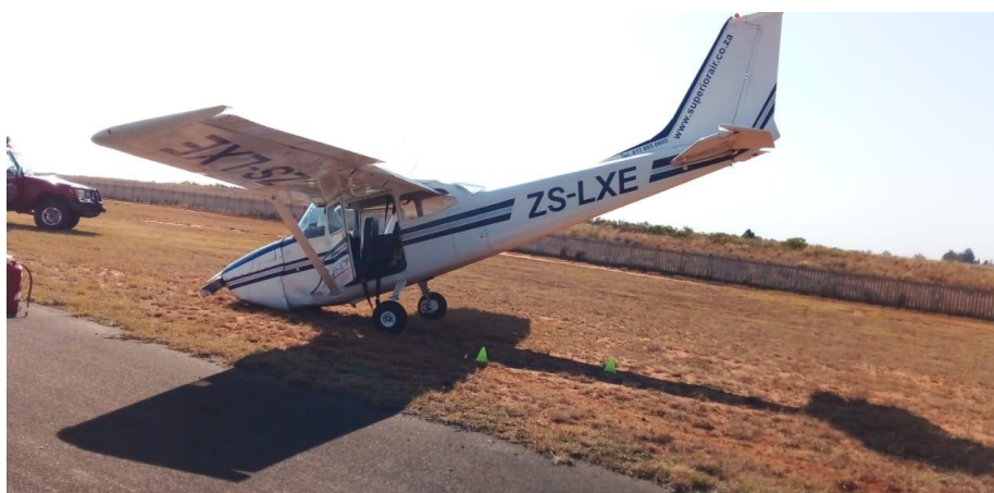
Figure 1: The aircraft next to Runway 35 with the flaps extended to 30°. (Source: Operator)
