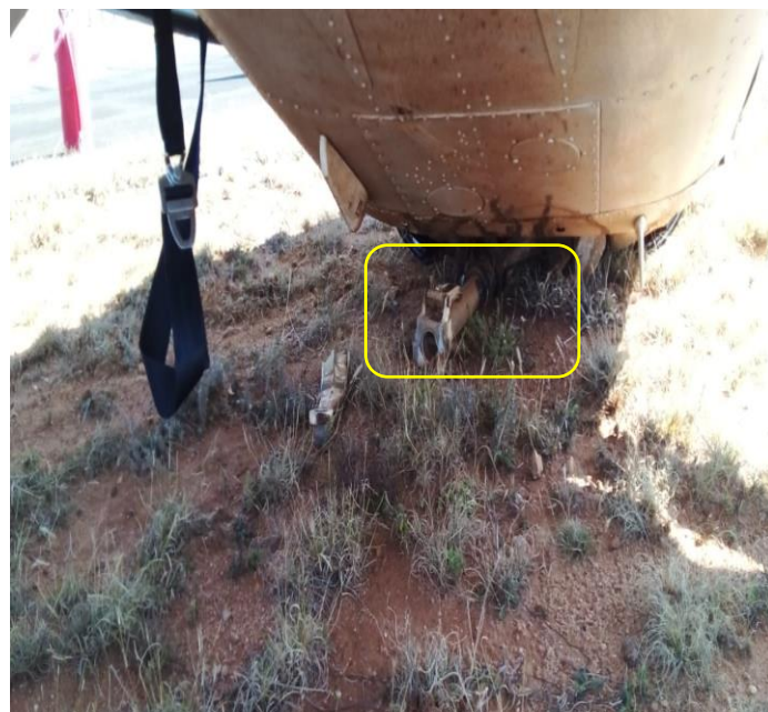
Figure 3: The rear of the aircraft showing a broken nose landing gear strut (yellow window). (Source: Pilot)
