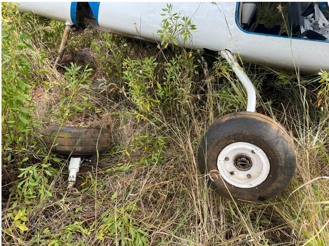
Figure 3: The left main landing gear that broke off. (Source: Operator)
