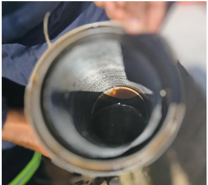
Figure 2: Traces of oil spillage mostly on the oil reservoir. Figure 3: The remaining oil in the reservoir was less than 100ml.
