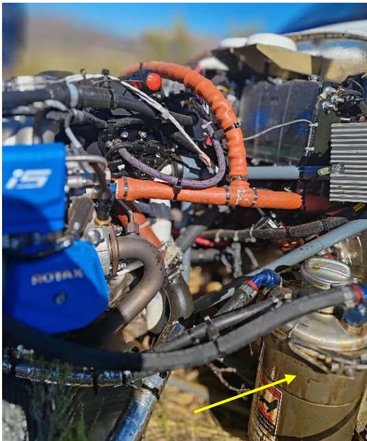
Figure 2: Traces of oil spillage mostly on the oil reservoir. Figure 3: The remaining oil in the reservoir was less than 100ml.
