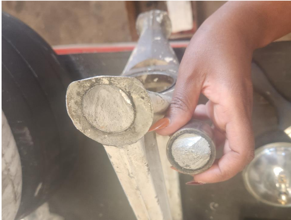
Figure 3: The broken left-side nose gear trunnion pin.
