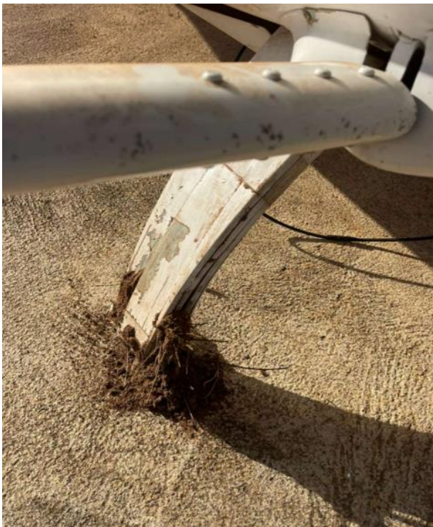
Figures 2 and 3: Shows the damaged right gear strut (left) and wheel assembly (right). (Source: Pilot)
