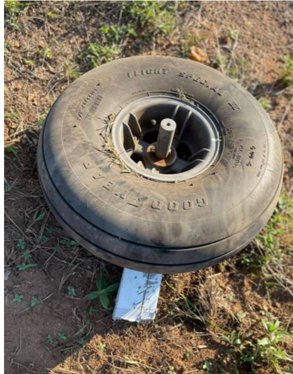
Figures 2 and 3: Shows the damaged right gear strut (left) and wheel assembly (right). (Source: Pilot)
