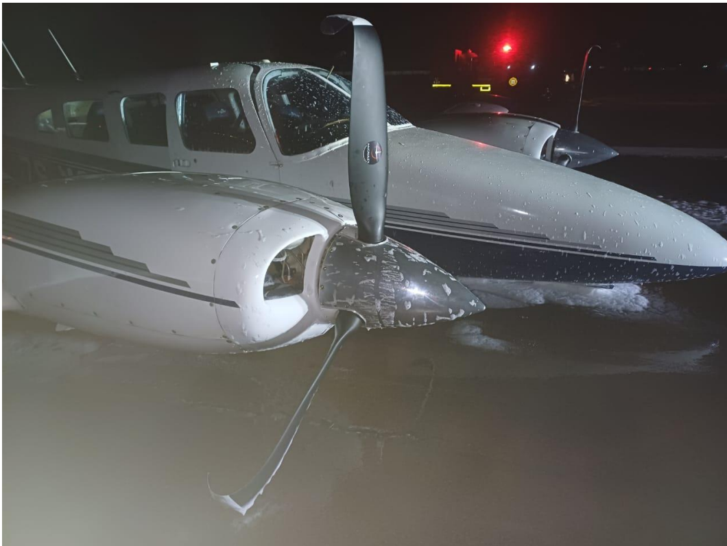
Figure 4: Damaged propeller blades and the scarred underbelly. (Source: Operator)
