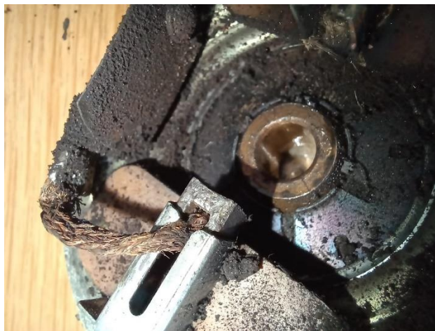
Figures 1 and 2: Oil deposits found inside the motor caused the brushes to soften and, thus, preventing proper contact.
