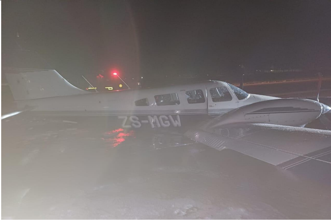
Figure 3: Foam applied to the runway after the aircraft had stopped. (Source: Operator)
