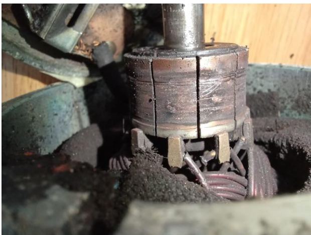
Figures 1 and 2: Oil deposits found inside the motor caused the brushes to soften and, thus, preventing proper contact.
