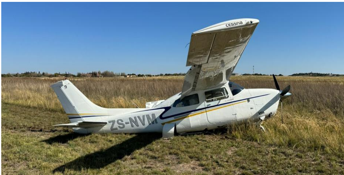
Figure 2: The aircraft as it came to rest after the accident with the nose gear extended. (Source: Pilot)
