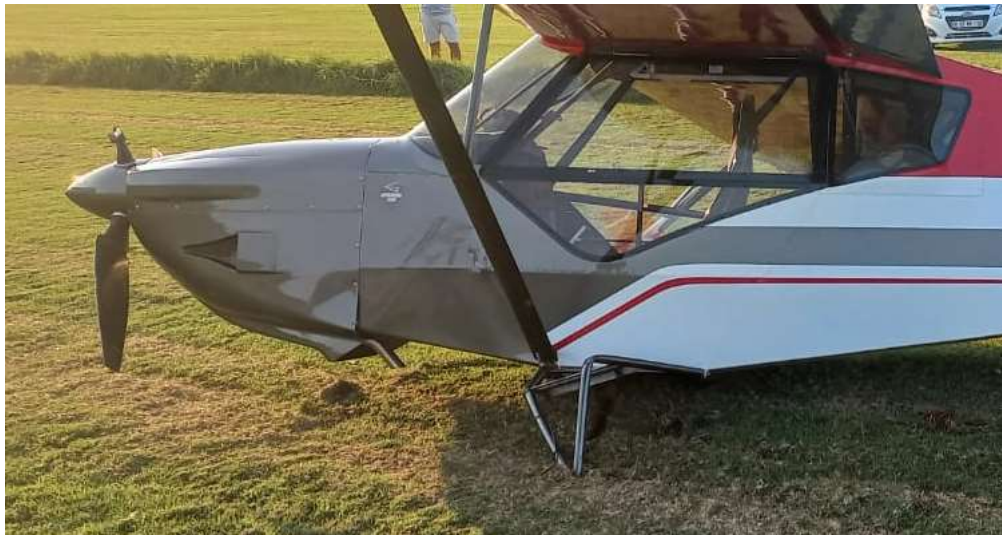
Figure 4: The bent left main gear strut, and the broken axle. (Source: Pilot)
