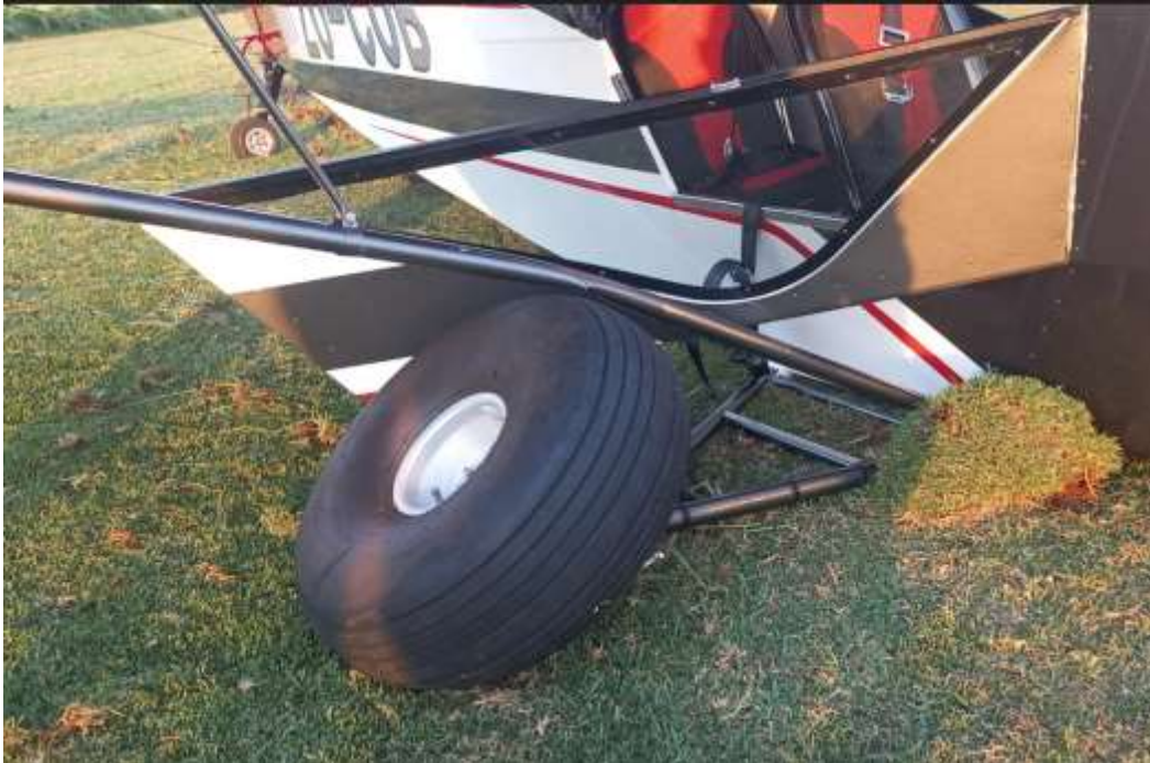
Figure 3: The right main landing gear strut that bent outward. (Source: Pilot).
