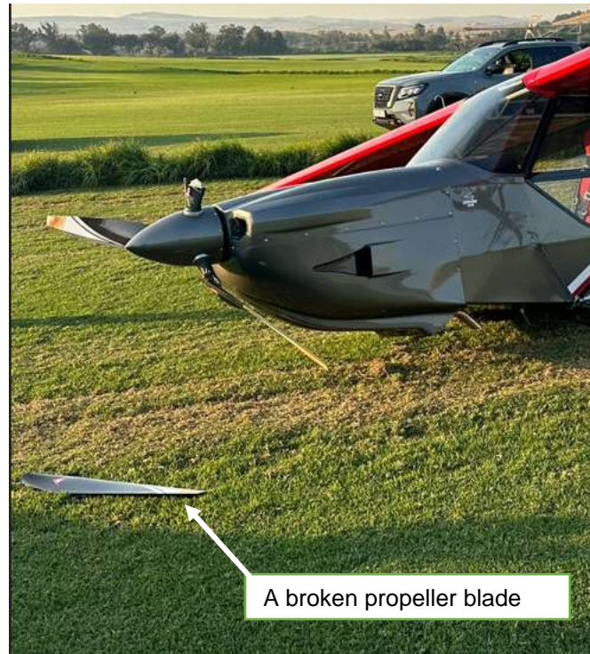
Figure 5: The propeller blade that broke off. (Source: Pilot).
