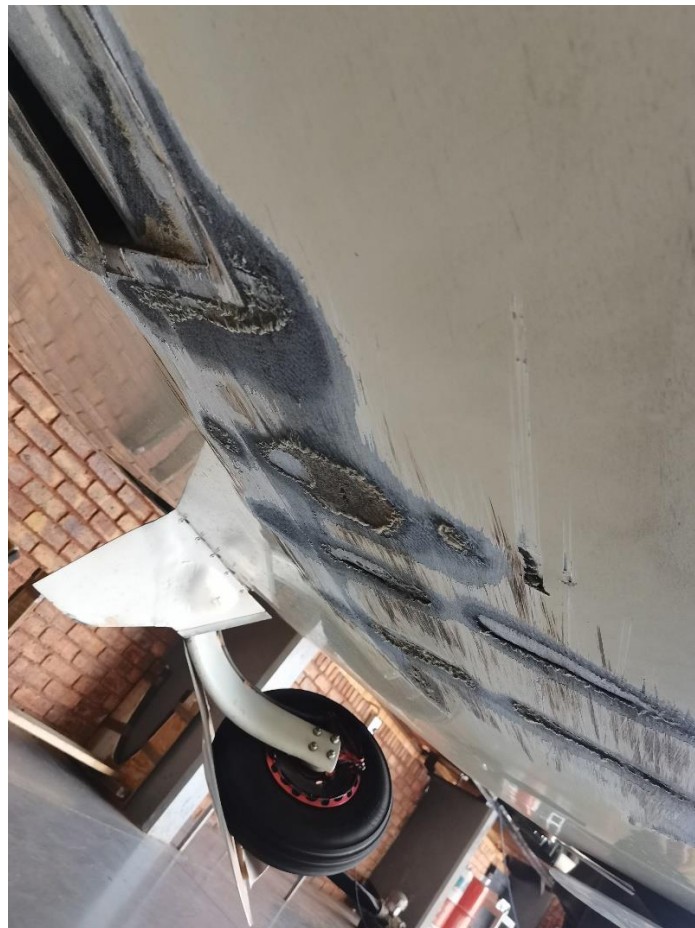
Figure 3: The damaged underbelly.
