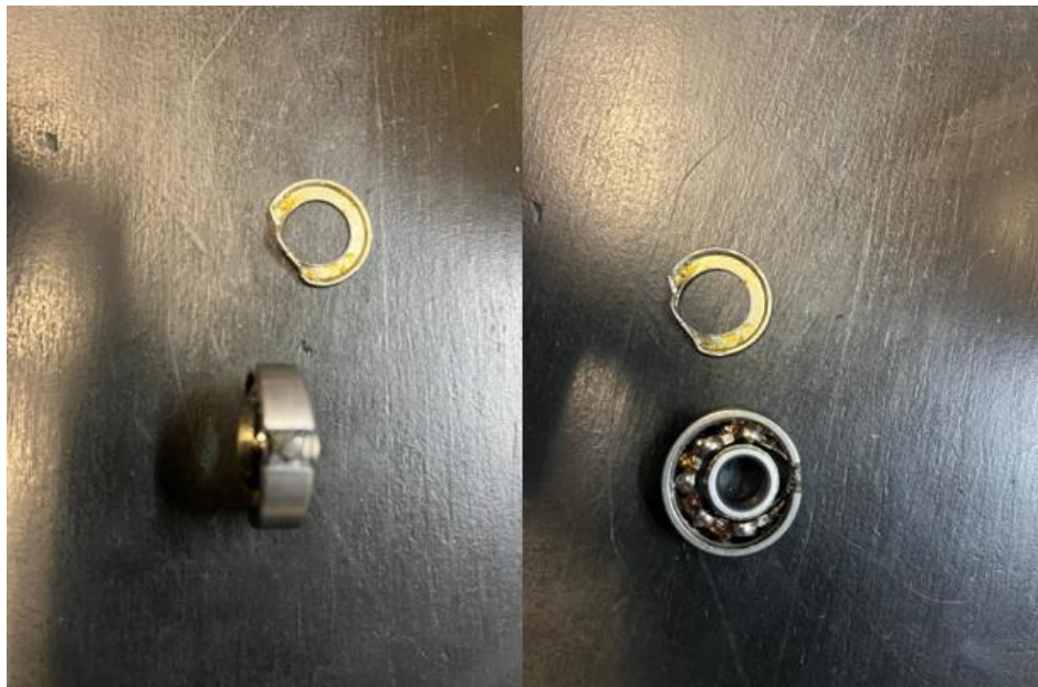
Figure 7: Damage to the bearing.
