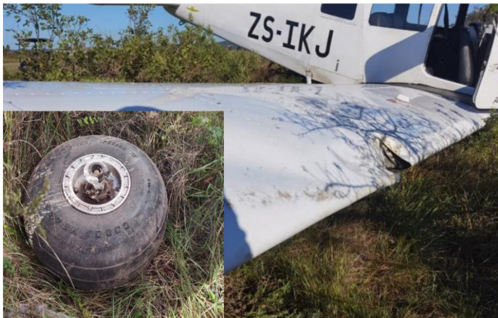
Figure 2: The nose gear that broke off and the damaged right-side wing. (Source: Operator)
