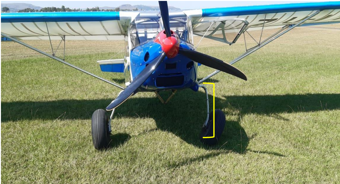
Figure 1: The aircraft at the accident site with a bent left main gear strut. (Source: Pilot)
