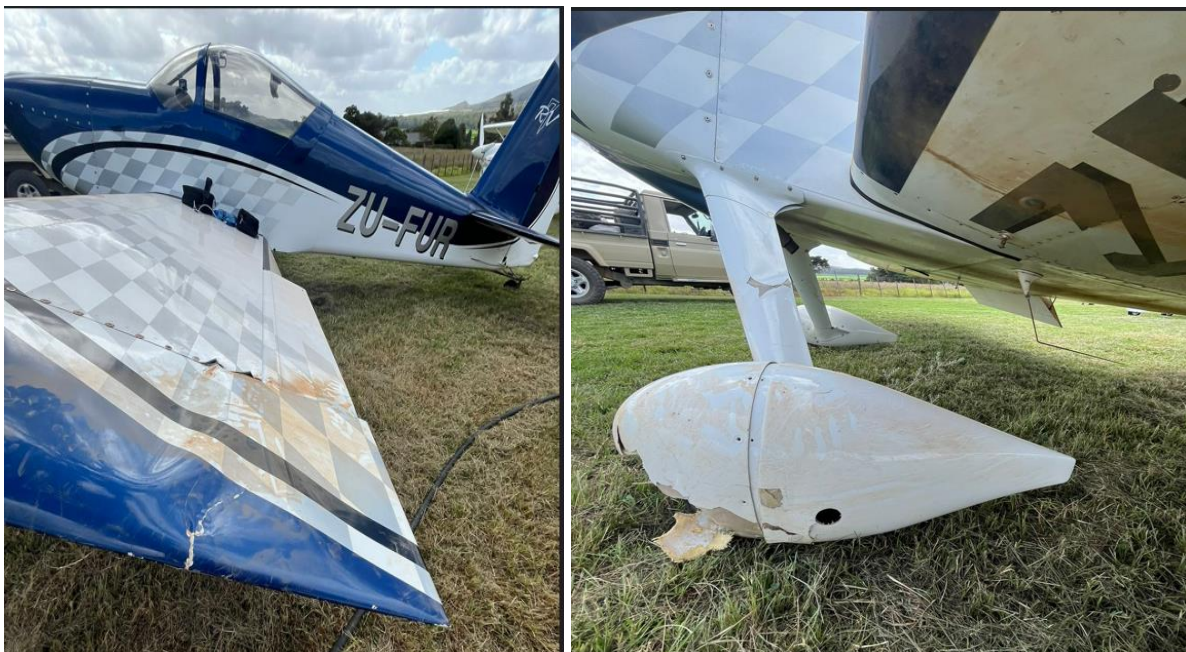
Figure 3: The damage sustained to the left wing (left picture). The damaged left main gear wheel fairing (right picture). (Source: Pilot)
