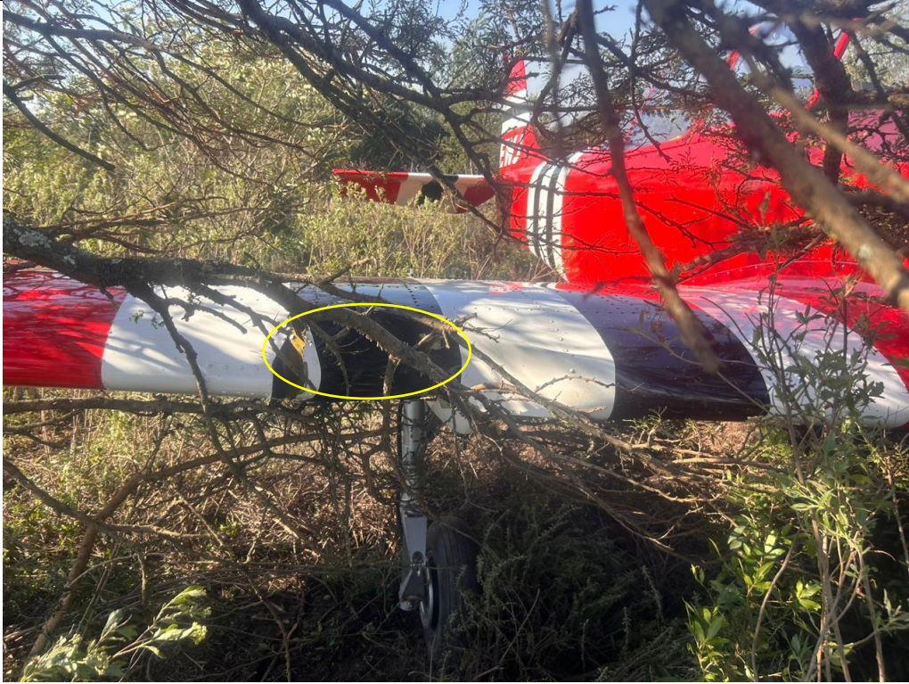
Figure 3: The damaged right wing (indicated in the yellow circle). (Source: Operator)
