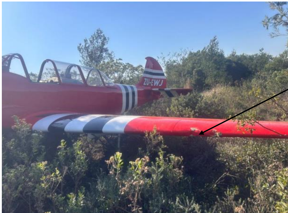
Figure 2: The dented left wing leading edge. (Source: Operator)
