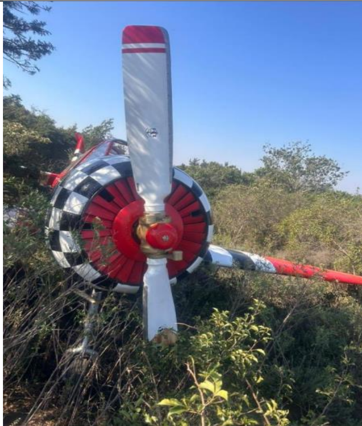
Figure 1: The damaged propeller. (Source: Operator)
