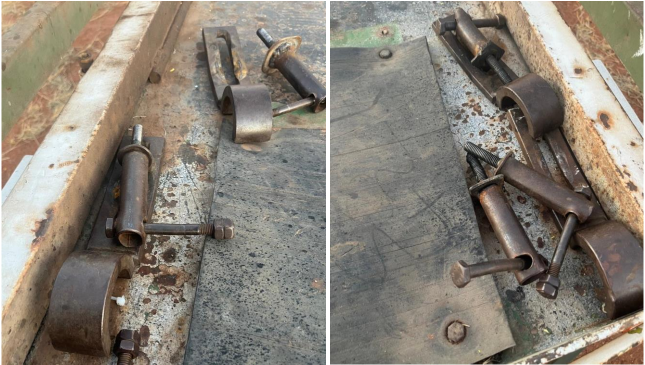
Figure 5: Some of the brackets used to secure the helicopter to the trailer. (Source: Pilot)
