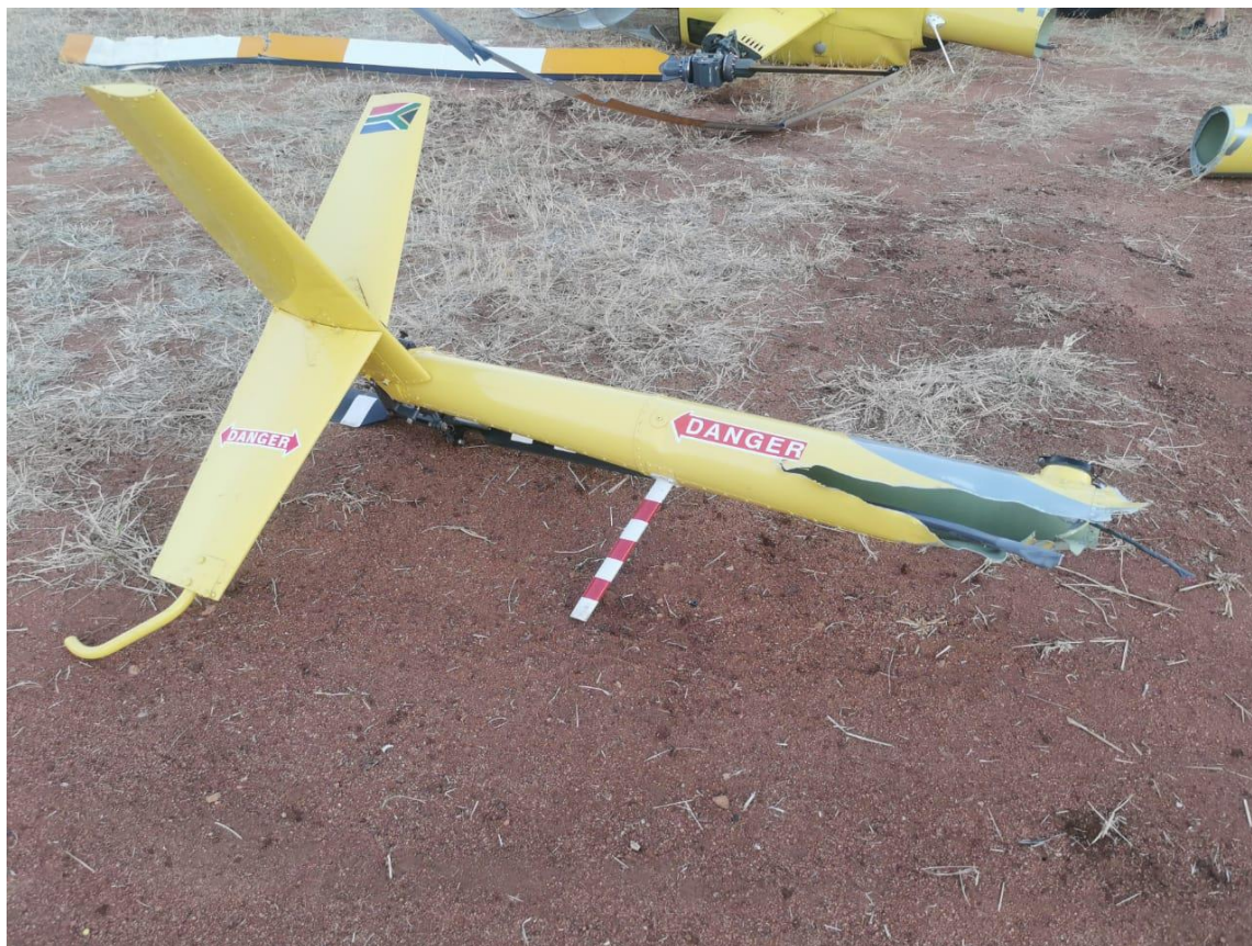
Figure 2: The tail boom was severed from the fuselage. (Source: Pilot)
