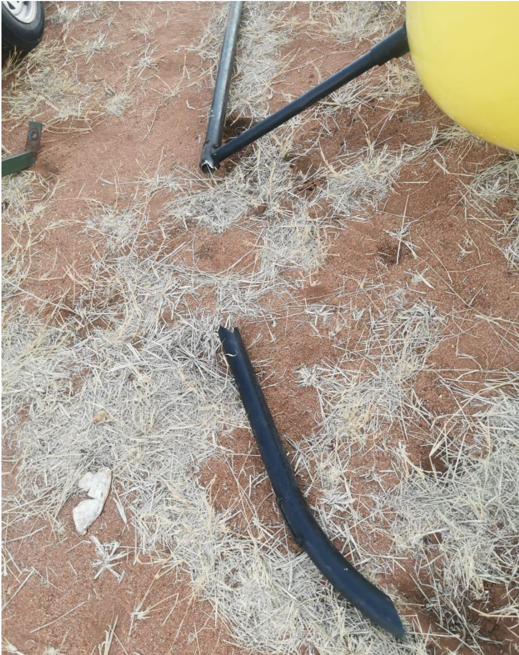
Figure 3: The left front section of the skid gear that broke off. (Source: Pilot)
