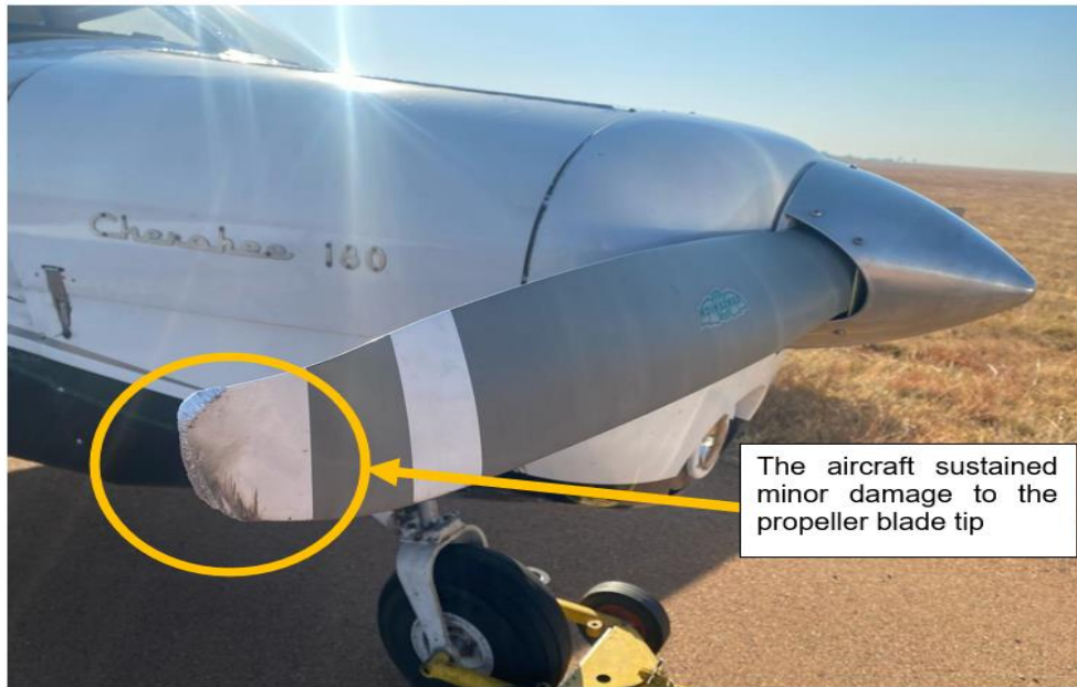
Figure 1: The damaged propeller blade. (Source: Operator)
