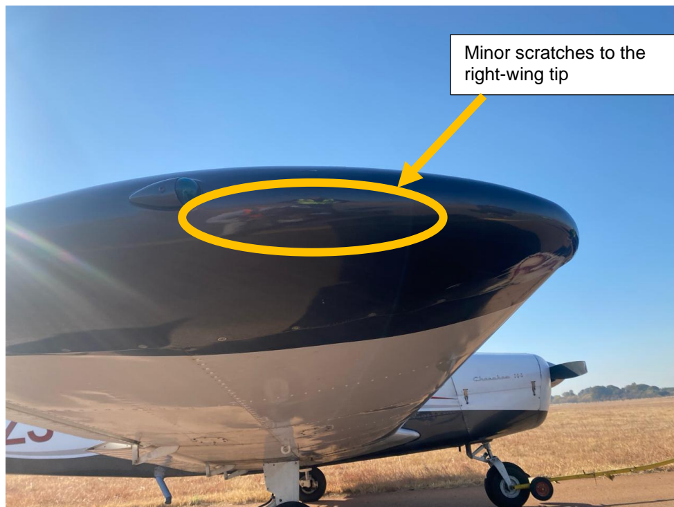
Figure 2: The right-wing tip with minor scratches. (Source: Operator)
