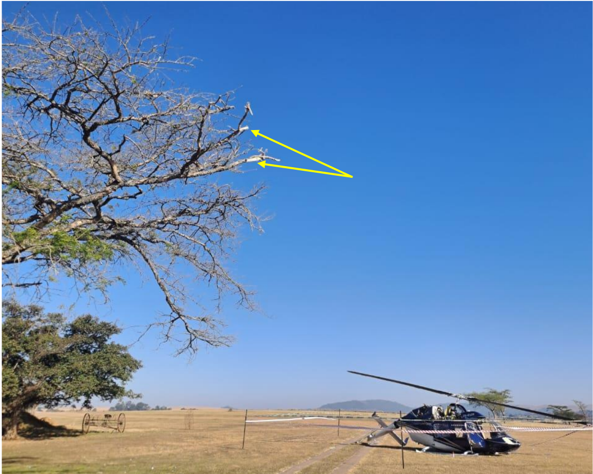
Figure 3: The helicopter and the tree branches struck by the main rotor blades. (Source: Pilot)
