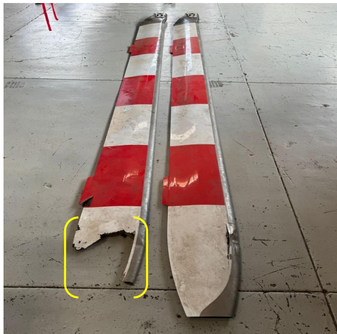
Figure 4: The severed main rotor blade tip. (Source: Pilot)
