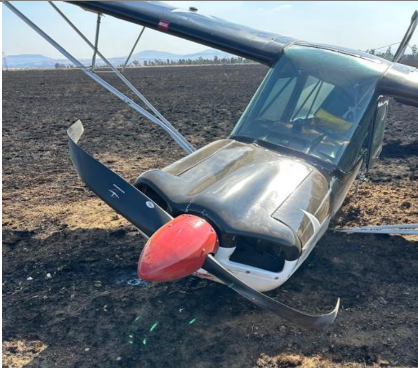
Figure 2: Front view of the aircraft with the damaged propeller blades. (Source: Operator)
