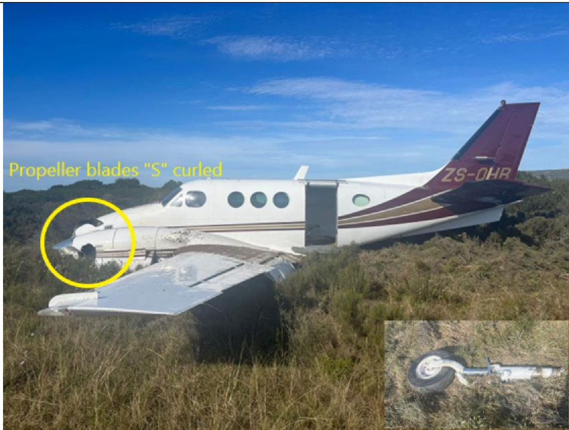
Figure 1: The aircraft came to rest facing north. Inset: The nose wheel gear that broke off. (Source: Owner)
