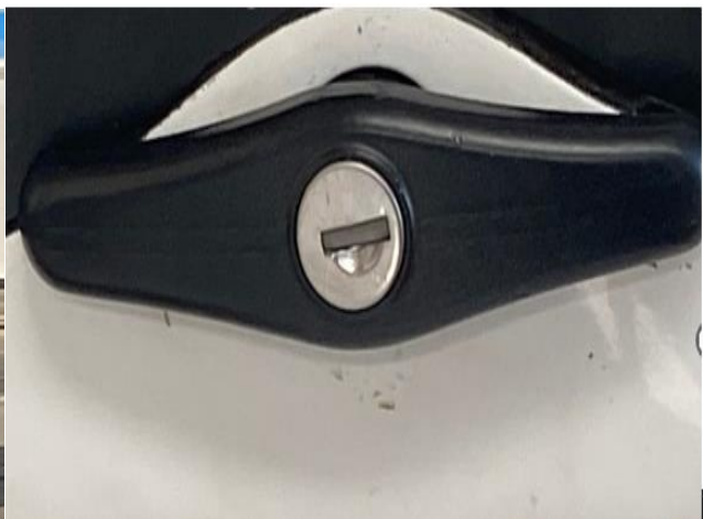
Figure 10: Correctly latched exterior door handle.
