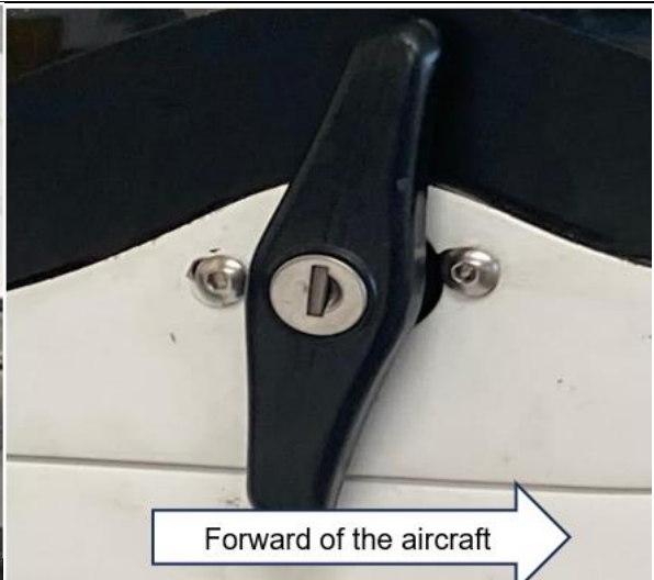
Figure 8: Improperly latched exterior door handle.
