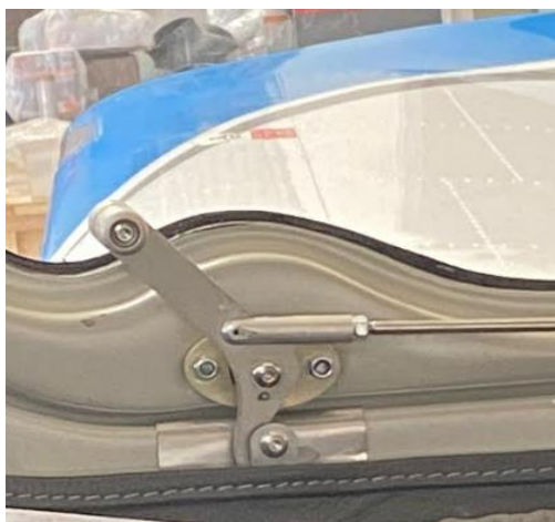
Figure 9: Correctly latched interior door handle.
