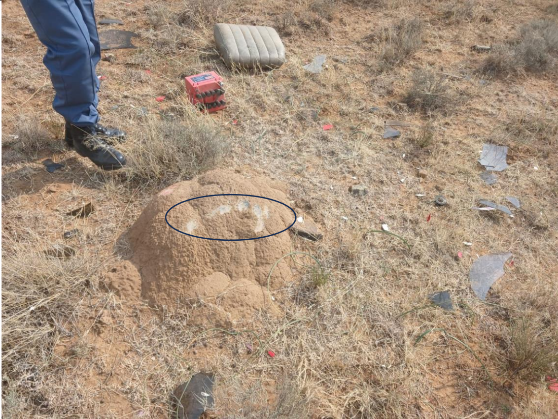
Figure 2: The tail rotor blades marks on the anthill. (Source: SAPS)
