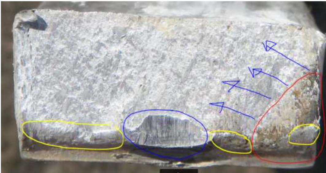
Figure 8: Fractures on the bracket surface.
