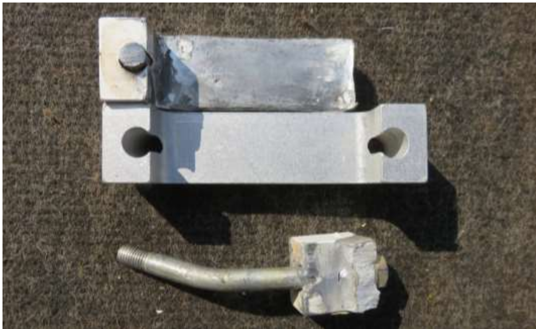
Figure 7: The picture depicts the fractured bracket and a new bracket.
