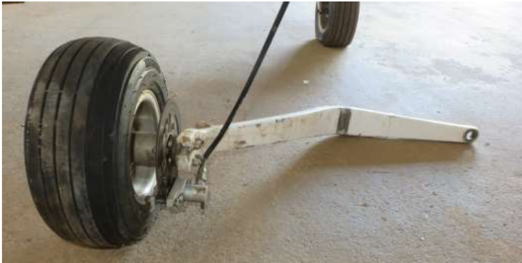
Figure 10: The undamaged left main gear leaf spring strut.
