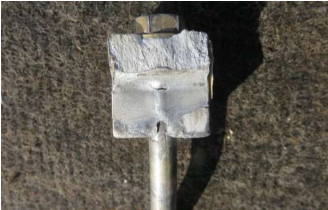
Figure 9: The bracket a with fractured surface.
