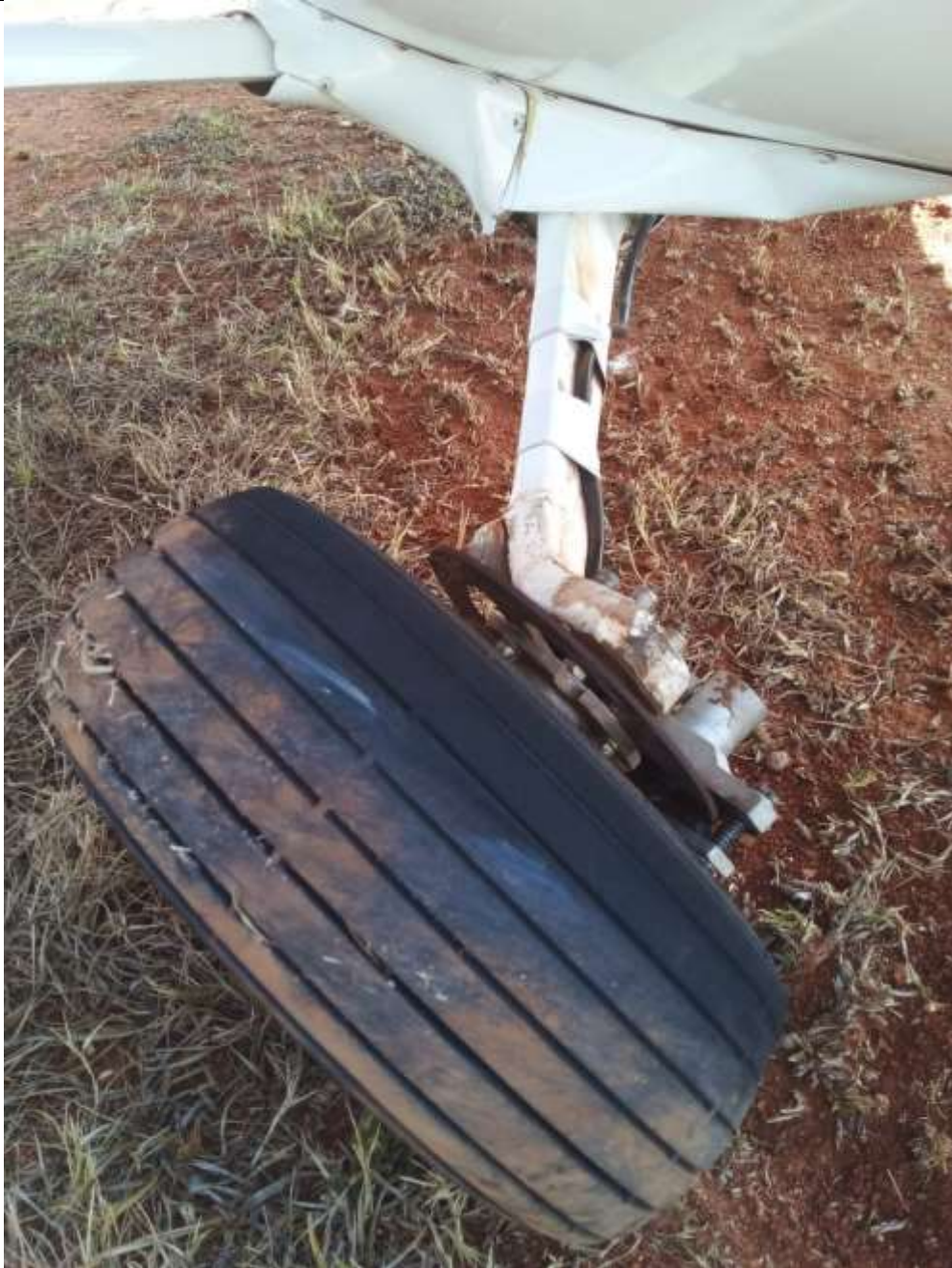
Figure 4: The left main landing gear leaf spring strut that folded backwards. (Source: Pilot)
