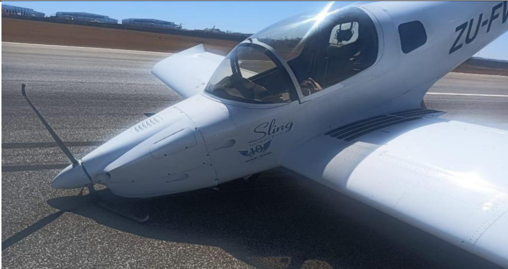
Figure 3: The damaged propeller. (Source: ARFF)
