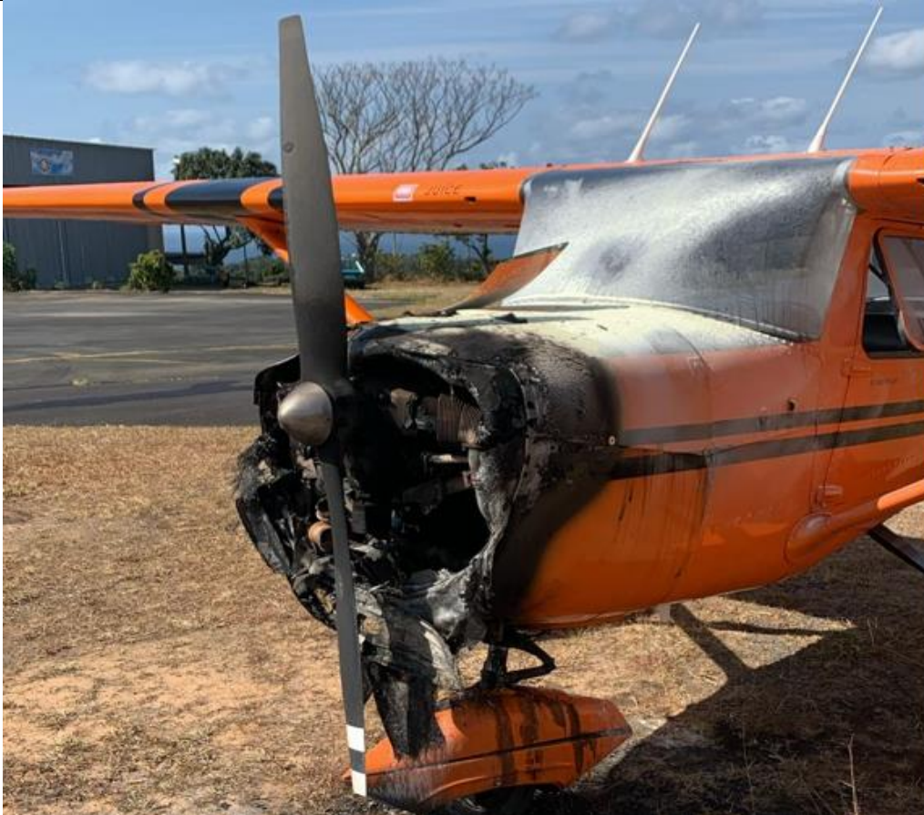
Figure 3: Damage in the engine section. (Source: Pilot)
