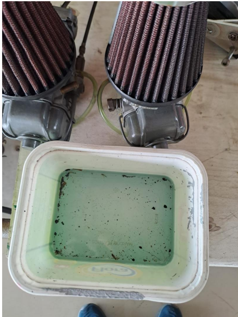
Figure 4: The filters and contaminated fuel. (Source: AP)
