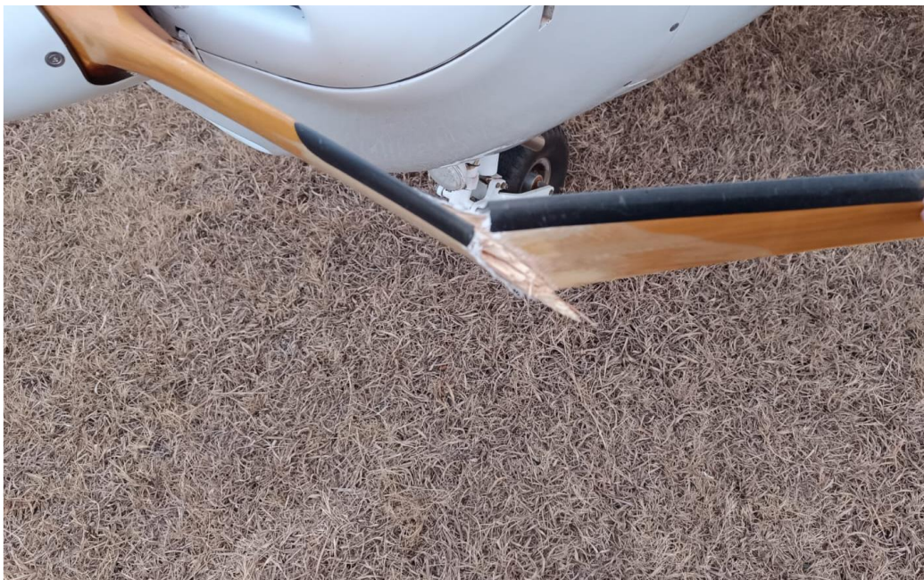
Figure 2: The damaged propeller blade. (Source: Owner)
