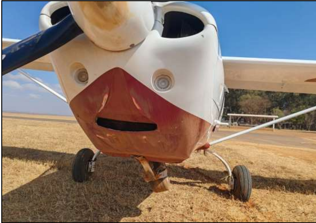
Figure 3: The collapsed nose landing gear strut after impact with the concrete edge of the taxiway. (Source: Operator)
