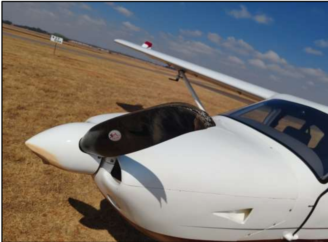
Figure 4: The damaged propeller spinner and blade tips. (Source: Operator)
