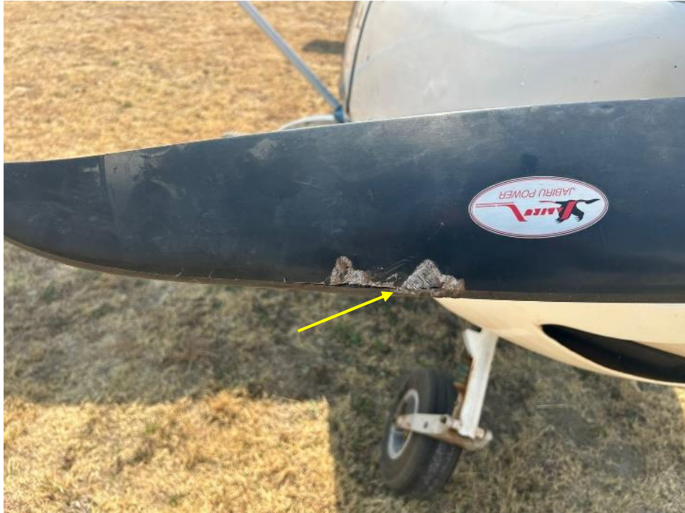
Figure 3: Damage on the composite propeller leading edge. (Source: Operator)
