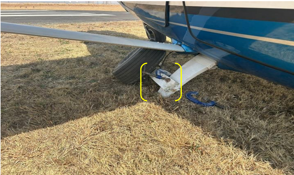
Figure 2: The aircraft with the broken left main gear. (Source: Operator)
