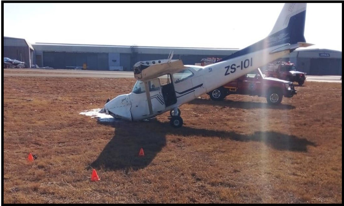
Figure 1: The aircraft as it came to a stop after exiting the runway. (Source: Owner)
