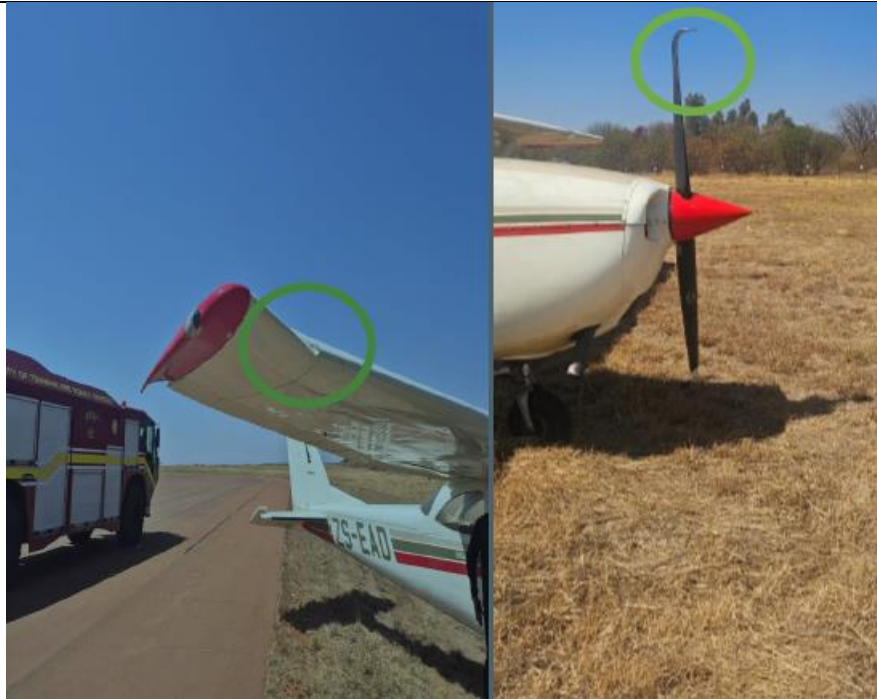
Figure 3: The aircraft sustained damage to the wing tip and the propeller. (Source: Pilot)
