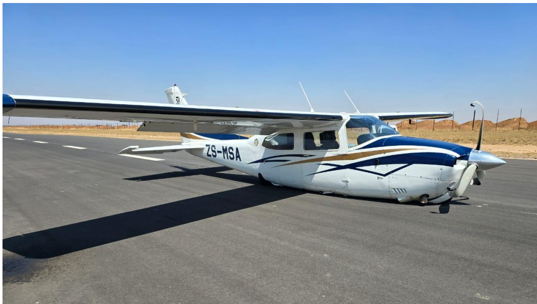
Figure 2: The aircraft after it had stopped on the runway with the landing gear retracted. (Source: Pilot)
