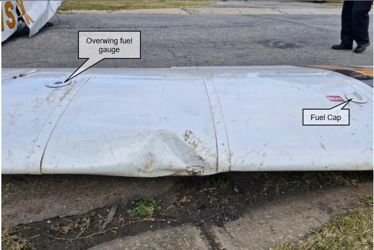
Figure 2: Damage from the initial impact with the first tree.
