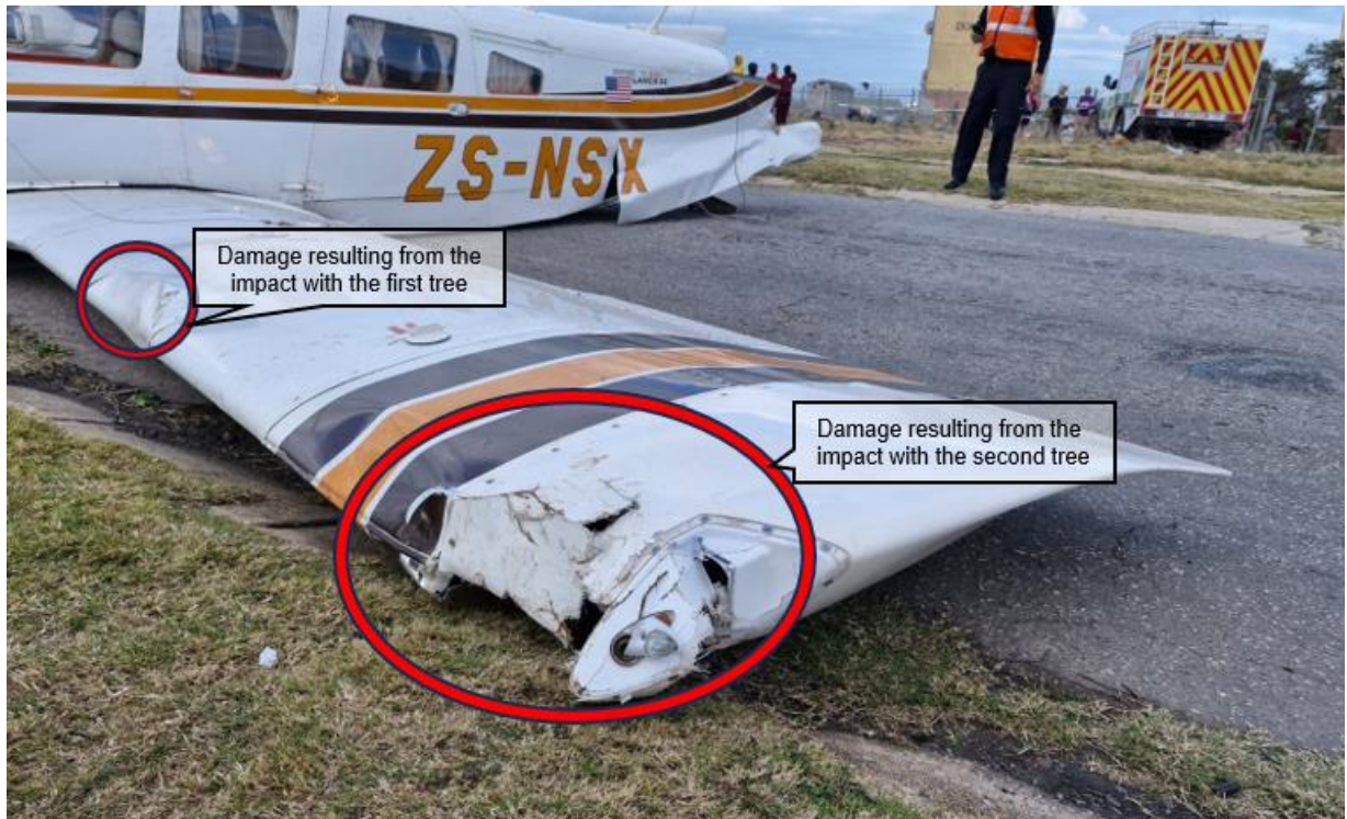
Figure 3: The damaged wing tip after the second impact with the tree.
