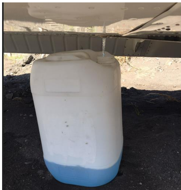
Figure 6: Approximately 5 litres of fuel was drained from the left tank.
