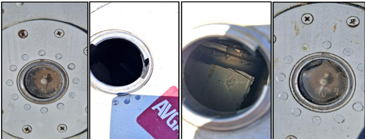
Figure 5: The left and right fuel tanks were empty, and the gauges indicated zero.
