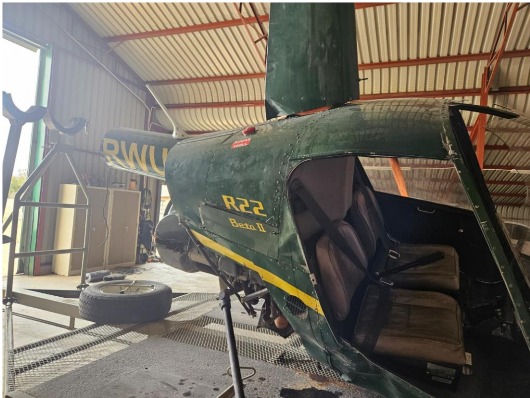
Figure 2: The helicopter rolled on to its right side during the accident. (Source: Pilot)
