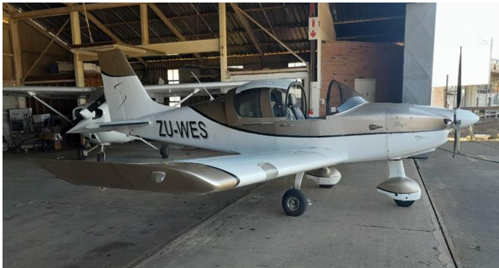
Figure 2: ZU-WES after recovery with the right main wheel fairing missing. (Source: Operator)
