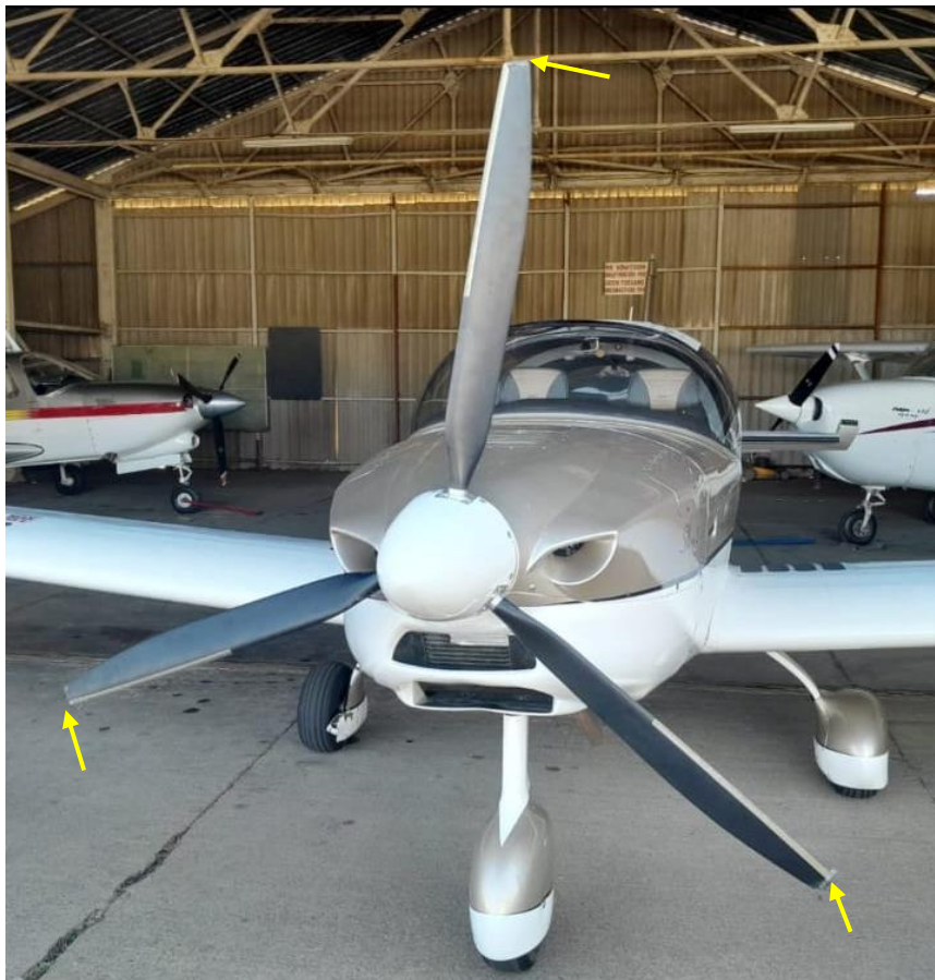
Figure 4: The damage on the propeller blade tips. (Source: Operator)
