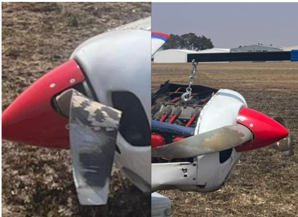
Figures 5 and 6: The bent propeller blades. (Source: Operator)
