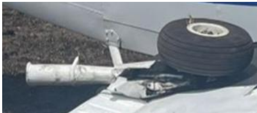
Figure 4: The right main landing gear strut. (Source: Operator)
