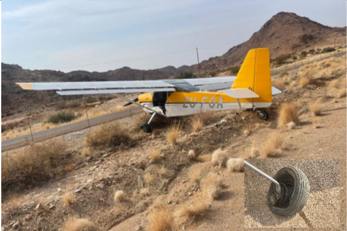
Figure 1: The aircraft stopped on the left side of RWY 01. The inset picture shows the damaged right-side tyre. (Source: Owner)
