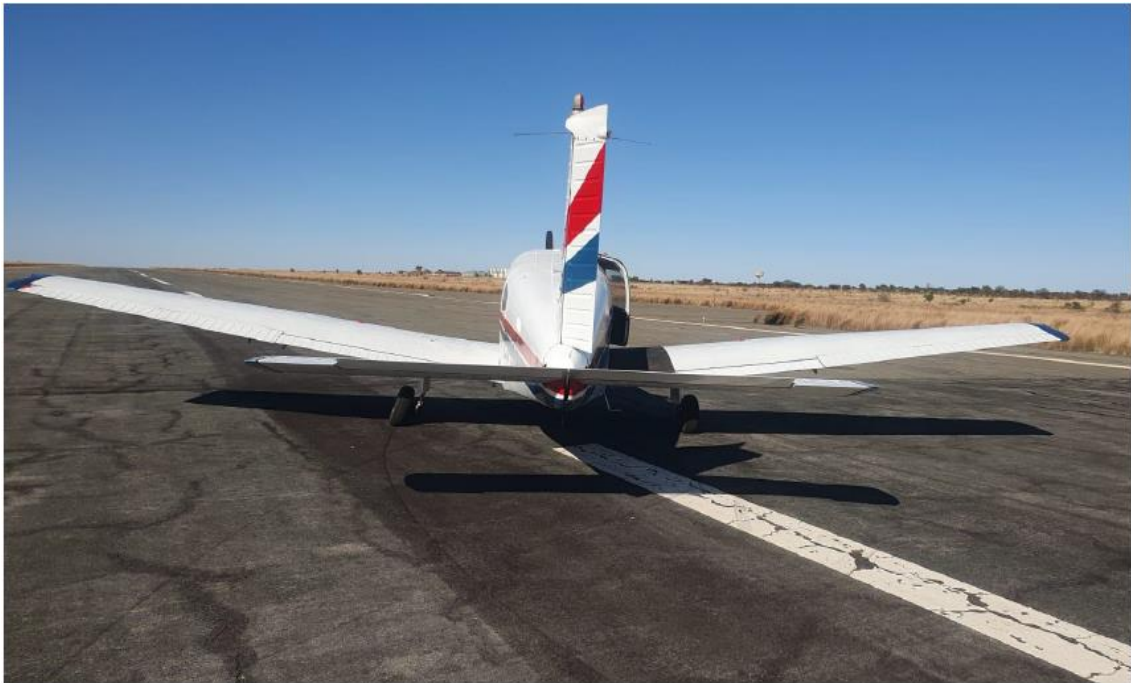
Figure 2: The damage on the left main undercarriage. (Source: Operator)
