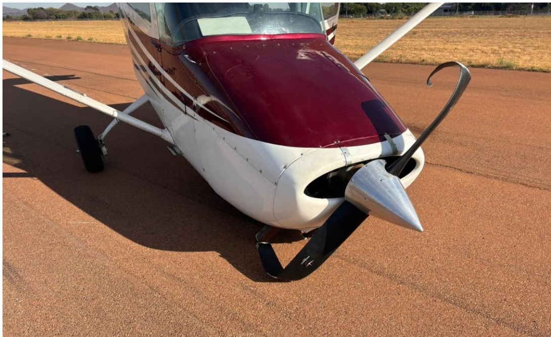
Figure 3: The deformed propeller blades indicate that the engine was delivering power during landing. (Source: ATO)
